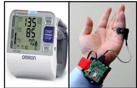
Figure 5: OMRON 7 series Wrist-watch Monitor (left), Blood Pressure Monitor developed by MIT (right)
