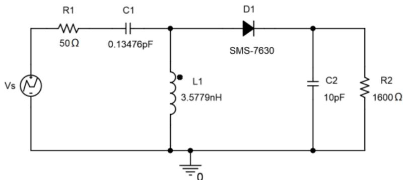
The output capacitor chosen as  $C2 = C_{out} = 100\text{pF}$  for  $B = 1\text{MHz}$
