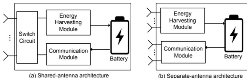
For enabling CSI acquisition, each ER must have a **communication module**, in addition to the **energy harvesting module**
