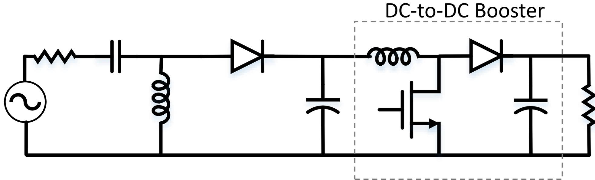
DC-to-dc boost voltage converter controls its input impedance (i.e: rectifier load  $R_L$ ) to set  $V_{dc}$  at the optimal value
