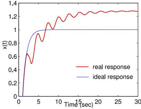
(a)  $Z$  is implemented as  $Z_b$  in the  $z$ -domain
