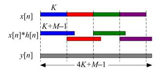
Each output chunk is of length K + M - 1 and overlaps the next chunk Operations:  $\approx \frac{N}{K} \times 8 (M + K) \log_2 (M + K)$ Computational saving if  $\approx 100 < M \ll K \ll N$
