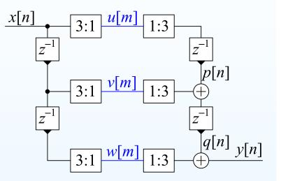
Input sequence x[n] is split into three streams at  $\frac{1}{3}$  the sample rate: u[m] = x[3m], v[m] = x[3m-1], w[m] = x[3m-2]
