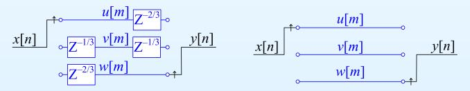
The commutator direction is against the direction of the  $z^{-1}$  delays.
