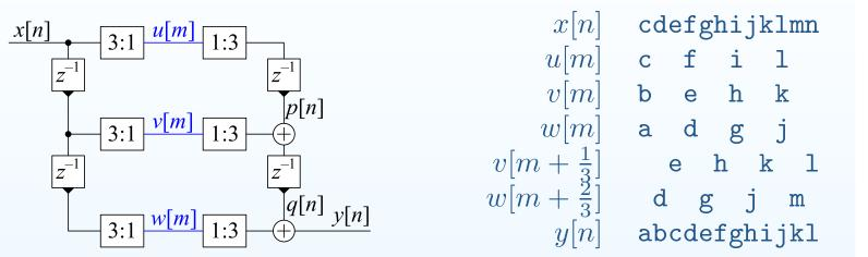
The combination of delays and downsamplers can be regarded as a commutator that distributes values in sequence to u, w and v. Fractional delays,  $z^{-\frac{1}{3}}$  and  $z^{-\frac{2}{3}}$  are needed to synchronize the streams. The output commutator takes values from the streams in sequence. For clarity, we omit the fractional delays and regard each terminal,  $\circ$ , as holding its value until needed.
