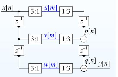
Input sequence x[n] is split into three streams at  $\frac{1}{3}$  the sample rate:
