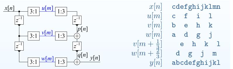
The combination of delays and downsamplers can be regarded as a commutator that distributes values in sequence to u, w and v. Fractional delays,  $z^{-\frac{1}{3}}$  and  $z^{-\frac{2}{3}}$  are needed to synchronize the streams. The output commutator takes values from the streams in sequence. For clarity, we omit the fractional delays and regard each terminal,  $\circ$ , as holding its value until needed. Initial commutator position has zero delay.
