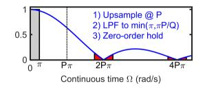
Equivalent to converting to analog with zero-order hold and resampling at  $f_y = \frac{P}{Q}$ .
