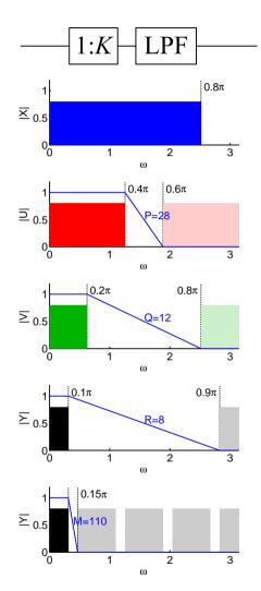
Alternative approach using direct 1:8 upsampling:  $\Delta \omega = 0.05\pi \Rightarrow M = 110 \Rightarrow 111 f_x$  multiplications (using polyphase) 13: Resampling
