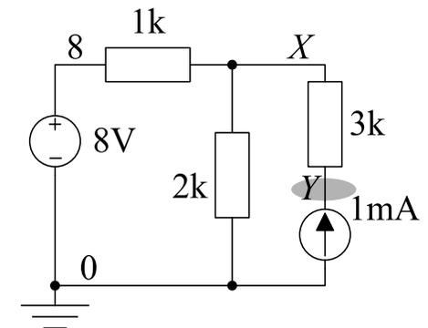
Ohm's law works OK if **all resistors** are in  $k\Omega$  and **all currents** in mA.
