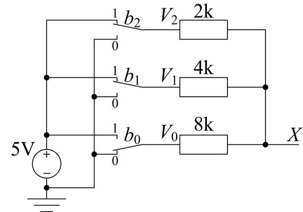
$$G_2 = \frac{1}{R_2} = \frac{1}{2} \text{ mS}, \dots$$
