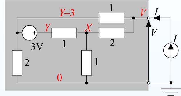
**Step 1:** Label ground as an output terminal + label other nodes.
