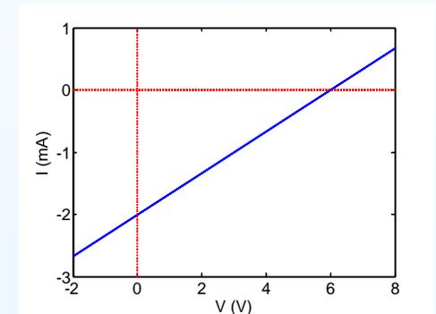
**Open Circuit Voltage:** If  $I = 0$  then  $V_{OC} = I_{No}R_{Th}$ .
