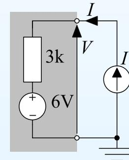
These four shaded networks are *equivalent* because the relationship between  $V$  and  $I$  is *exactly* the same in each case.
