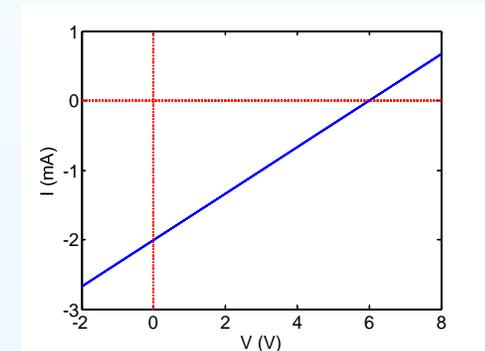
Open Circuit Voltage: If  $I = 0$  then  $V_{OC} = I_{No} R_{Th}$ .
