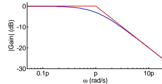
A *low-pass* filter because it allows low frequencies to pass but *attenuates* (makes smaller) high frequencies.
