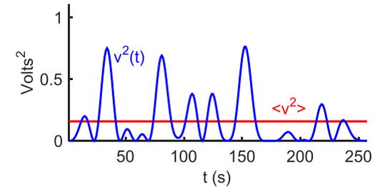
*Instantaneous Power* dissipated in  $R$ :  $p(t) = \frac{v^2(t)}{R}$
