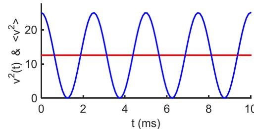
*Cosine Wave:*  $v(t) = 5 \cos \omega t$ . Amplitude is  $V = 5$  V.
