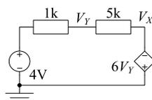
13. [C] Find the equivalent resistance of the network shown below.
