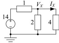
2. [B] Calculate  $V_X$  and  $I_X$  in the following circuit using (a) nodal analysis and (b) simplifying the circuit by combining parallel resistors.
