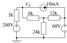
6. [C] Calculate  $V_X$  in the following circuit.
