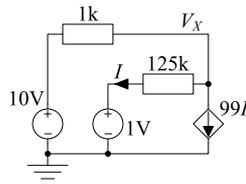
8. [C] In the following circuit calculate  $V_X$  in terms of  $V$  and  $I$  using (a) nodal analysis and (b) superposition.
