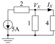
3. [C] Calculate  $V_X$  in the following circuit using (a) nodal analysis and (b) superposition.
