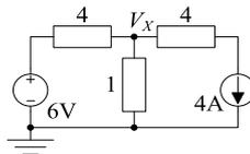
4. [C] Calculate  $V_X$  in the following circuit.
