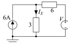
11. [C] Calculate  $V_X$  in the following circuit using (a) nodal analysis and (b) superposition.
