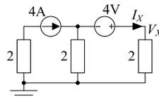
10. [C] Determine an expression for  $I_X$  in terms of  $V$  in the following circuit. Determine the value of  $V$  that will make  $I_X = 0$ .
