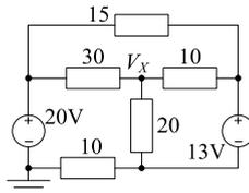
5. [C] Calculate  $V_X$  in the following circuit.
