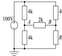
15. [D] Calculate  $V_X$  in the following circuit. You can either use nodal analysis directly or else simplify the circuit a little to reduce the number of nodes.
