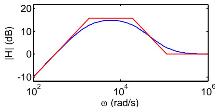
The high frequency asymptote has a gain of 1 (as is clear from the circuit in any case). Since the two highest corner frequencies differ by a ratio of 6, it follows that the gain of the central flat portion of the approximate magnitude response is also  $\left| \frac{Y}{X} \right| = 6 = 15.6 \text{ dB}$ . Alternatively, you can substitute  $\omega = \frac{0.1}{RC}$  into the low frequency asymptote expression:  $60j\omega RC$ . [3C]
