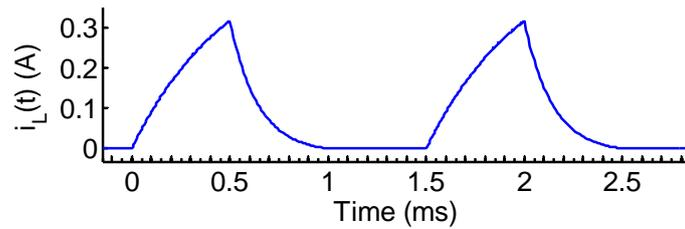
Many people thought the current would go negative and almost reach the steady state of  $-10\text{mA}$ . In fact, as soon as the current reaches zero, the diode turns off and the current stays at zero.
