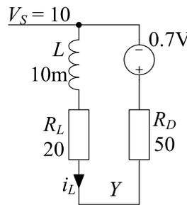
The time constant is therefore  $\tau_O = \frac{L}{R_L + R_D} = 0.143 \text{ ms}$  and the steady state current is  $I_O = \frac{-0.7}{R_L + R_D} = \frac{-0.7}{70} = -10 \text{ mA}$ .
