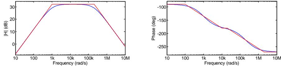
For the magnitude plot the corners are at  $\left(\frac{1}{R_1C_1}, \frac{R_2}{R_1}\right)$  and  $\left(\frac{1}{R_2C_2}, \frac{R_2}{R_1}\right)$ .
