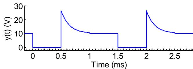
Quite a few people misread the question and drew a graph of  $i_L(t)$  instead. When the switch is open, you can calculate the voltage at  $Y$  relative to the  $10\text{V}$  supply in two ways (i) the sum of the voltages across the diode and the  $50\Omega$  resistor or (ii) the sum of the voltages across the inductor and the  $20\Omega$  resistor. The second way is much more effort because it depends on the derivative of the current; some people tried to do it this way nevertheless.
