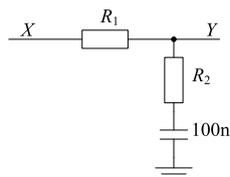
The transfer function of this network is  $\frac{R_2 + \frac{1}{j\omega C}}{R_1 + R_2 + \frac{1}{j\omega C}} = \frac{j\omega R_2 C + 1}{j\omega(R_1 + R_2)C + 1}$ . The LF and HF asymptotes are 1 and  $\frac{R_2}{R_1 + R_2}$  respectively, from which  $R_1 = 9R_2$ . The
