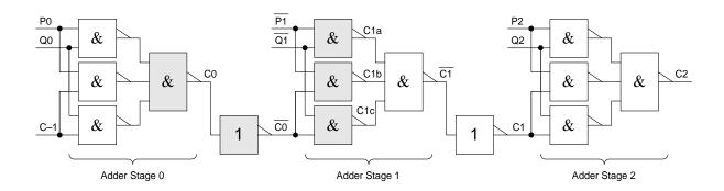
By merging the shaded gates we can reduce the delay to one gate per adder stage.
