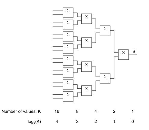
Each column of adders adds a delay of 6 and halves the number of values needing to be added together.
