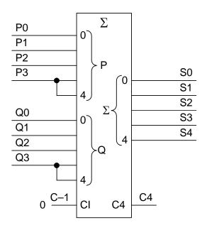
This is different from the unsigned case because P4 and Q4 are no longer constants. <u>We cannot simplify this circuit</u> by removing the MSB stage.
