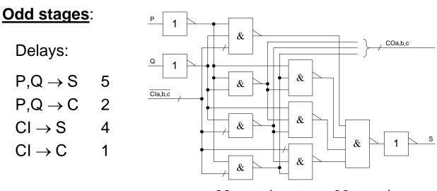
33 gate inputs  $\Rightarrow$  66 transistors
