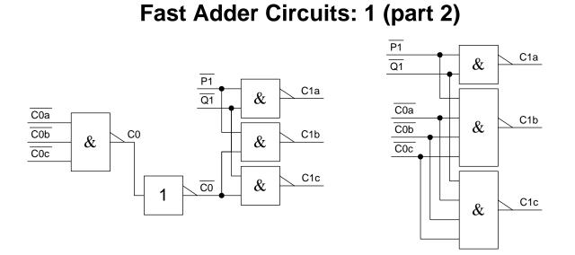
We can merge the 3-NAND and inverter into the final column of gates as shown; this gives one delay per stage:
