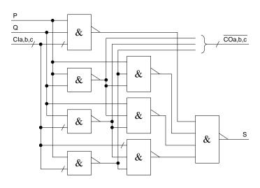
30 gate inputs  $\Rightarrow$  60 transistors
