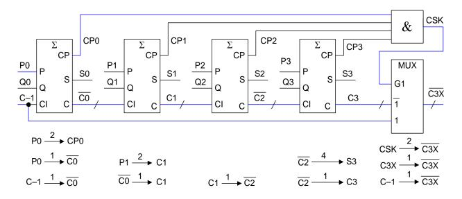
Calculate Carry Propagate (CP =  $P \oplus Q$ ) for each bit. Call this 2 gate delays since XOR gates are slow. CSK=1 if all bits propagate the carry.
