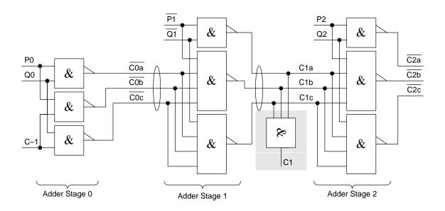
The signals C1a, C1b, C1c form an *AND-bundle*: C1 is true only if all of them are high. We don't need the signal C1 directly so the shaded gate can be omitted.
