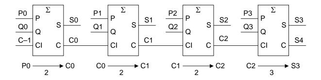
Delays within each stage (in gate delays):
