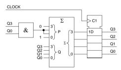
6C. Modify the above circuit so that it follows the count sequence 1, 2, 3, ..., 9, 10, 1, 2, 3, .... Draw a state diagram for your revised circuit.
