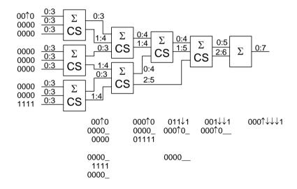
By inserting inverters between stages, we can change the delay to  $4 \times 2 + 6 = 14$ . We should not insert an inverter in the signal path that skips a stage.
