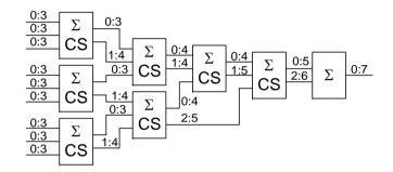
The SUM output from a CS adder must go from the lowest bit position of any input to the highest bit position of any input. The CARRY output must go from one more than the lowest bit position with at least two inputs to one more than the highest bit position with at least two inputs. This is because we need at least two inputs to generate a carry.
