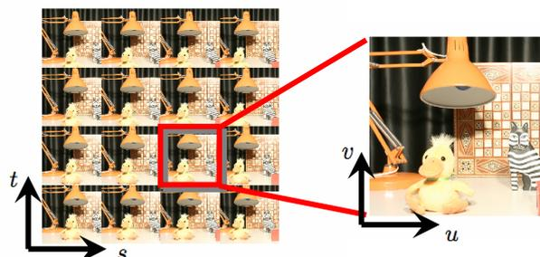
**Figure 3: The lightfield parameterisation.** The planar camera array shown in Figure 2 leads to the 4-D lightfield shown above. Here, the  $t,s$  coordinates correspond to the camera locations, while the  $u,v$  coordinates corresponds to the image plane
