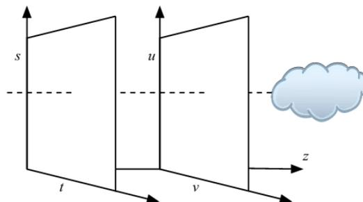
**Figure 1: 4D light field (or light slab) parameterization.** A light ray is uniquely characterised by its intersection between the camera plane  $(s,t)$  and the image plane  $(u,v)$ . Each light ray is therefore addressed by its coordinate  $(u,v,s,t)$
