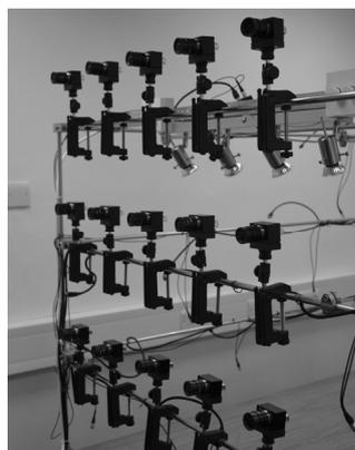
**Figure 2: Planar camera array.** (Note that this multi-camera system is supported by SEAS-DTC and The Royal Society)
