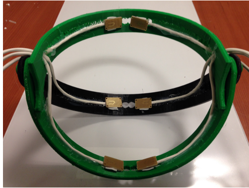
Figure 5: Differential electrode positioning in the headset for optimum P300 detection
