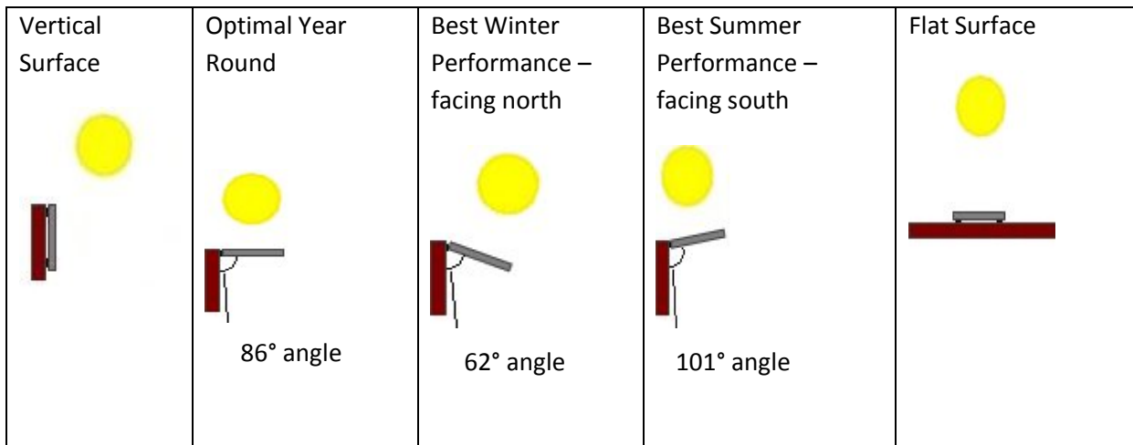
Fig. 3. The various positions of a panel with respect to the vertical surface that were considered.
