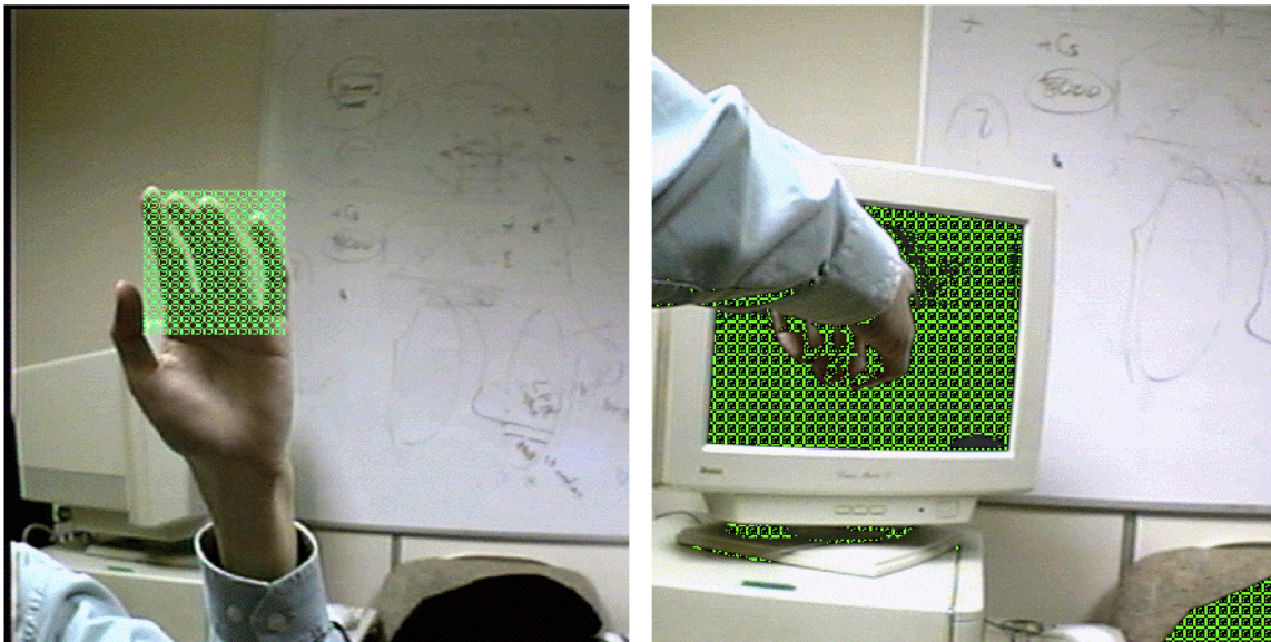
Figure 9 An example of motion-guided effects. The picture on the left shows a synthetic image whose size, position and pattern are controlled by the motion of the hand. The picture on the right shows an instant when the hand movement triggers an event. The corresponding operation is to surface map a given pattern on all images that are detected black in colour: these include the monitor screen and the object at the bottom right-hand corner.
