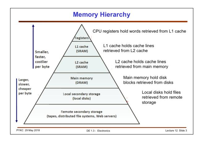
In any computer systems, storage of information is always organiised in a hierarchy as shown here as a triangle. This has many layers representing different type of storage.
