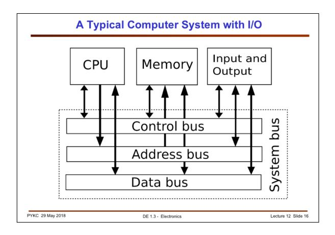
All these are interconnected via system buses: the address bus, the data bus and the control bus.
