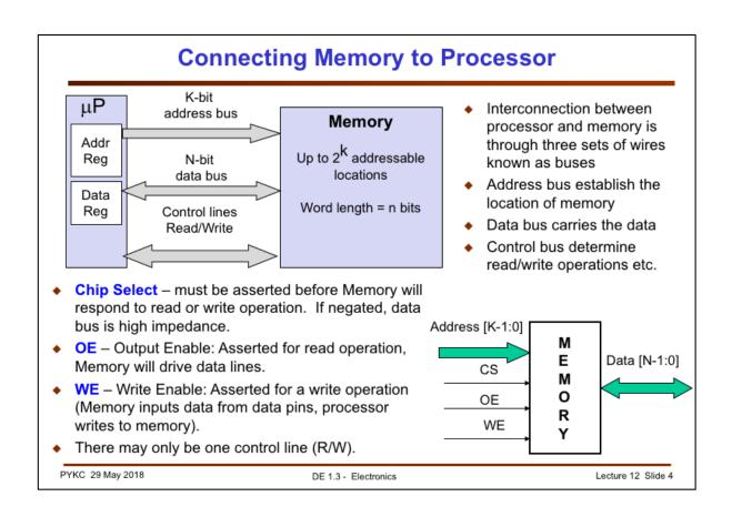
Memory chips (not cloud storage or disks) are connected to the microprocessor through three bundles of signal connections. These are called "buses".
