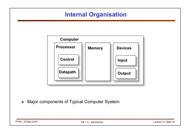
Here is a typical internal view of a computer. It has the processor (CPU), memory system (including disk storage) and input/output devices.
