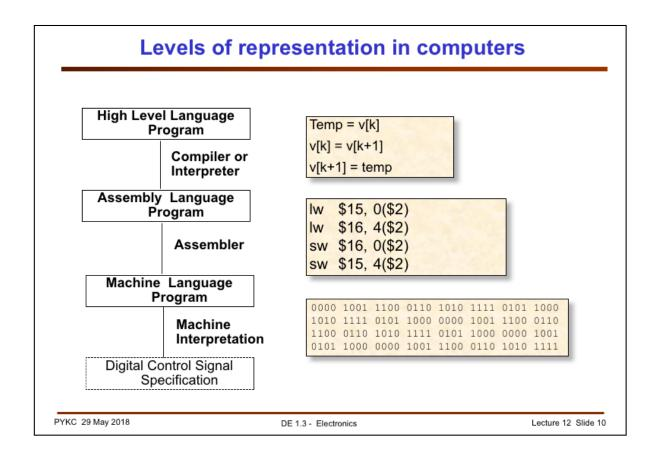
Here is diagram showing how a high level language is used to specify instructions to the CPU. It goes through different steps. First there is the compiler which produces lower level language (usually called assembly language programs). This is then translated to machine instructions in binary form. These instructions are decoded by the CPU to become digital signals that control gates and flip-flops on chip itself.
