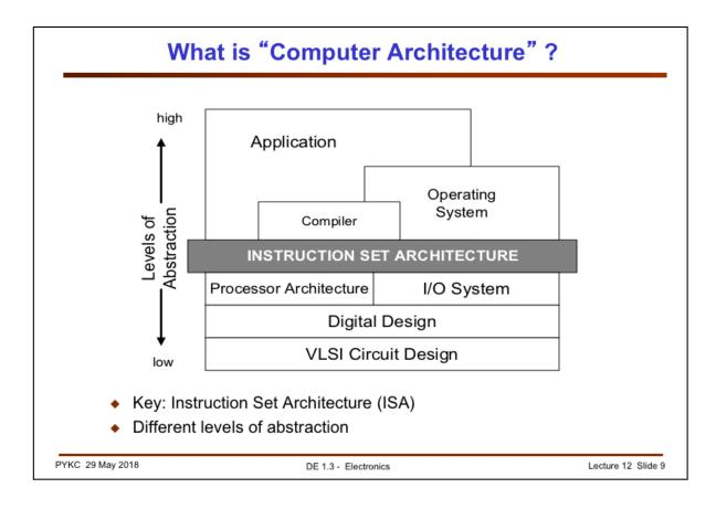
Now let us examine what makes up a computer system. Shown here is a hierarchy diagram from transistor level hardware (VLSI circuits) to the application programs. What is important is to appreciate the **levels of abstraction** used to present the system for different specialty of engineering.
