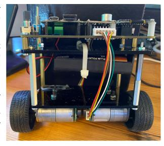
**Step 3**: Tuning the PID controller is difficult. I suggest that you hang the segway with some elastic cord that will be provided for you in Week 9, so that you can tune the segway without it falling over all the time.
