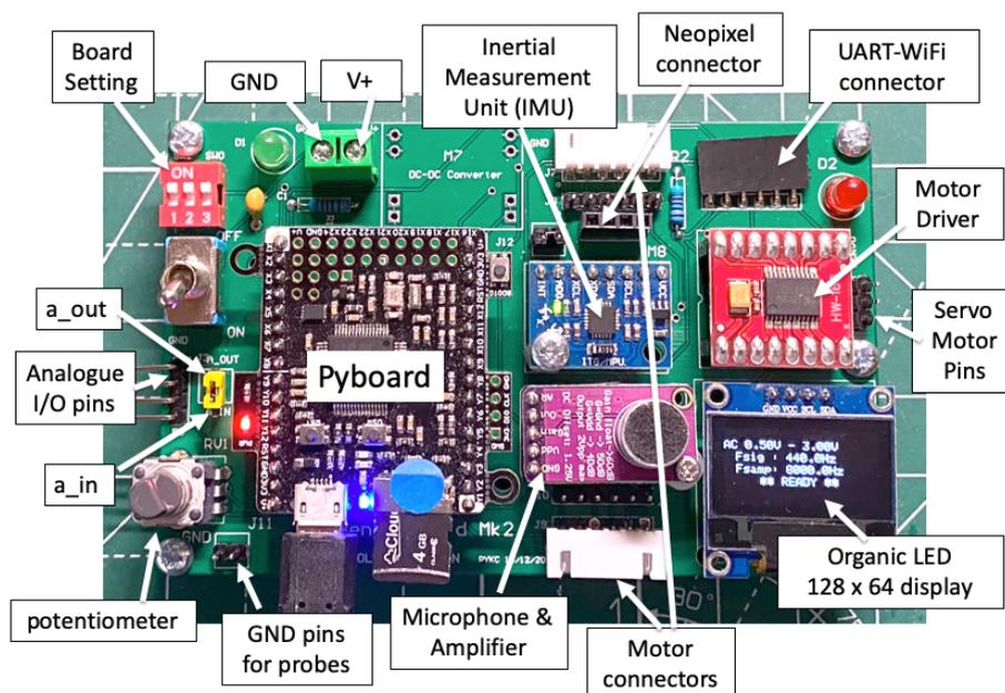
Unlike Electronics 1, you are **not** required to build electronics circuits on breadboard this year. Instead, you will be using a bespoke board (PCB) that I designed specifically for this module. This unit is known as **PyBench Board** – it is my version of an electronic workbench which is programmed using MicroPython (uPy), and controlled via the USB serial port.
