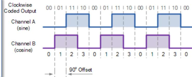
Each motor is equipped with two Hall effect sensors, which detect changes in magnetic field strength as shown in the photograph. The circular magnet has 13 pairs of N-S poles. The gear ratio of the motor is 1:30. This causes the hall effect sensors to produce  $13 \times 30 = 390$  square pulses per revolution of the wheel. Since the two sensors are slightly offset from each other, the square waves from the two sensors are at different phase angles.
