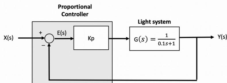
This question tests students understanding of feedback control systems. It particular tests for understanding of proportional control and its ability to reduce the impact of the error in the forward gain of a system.
