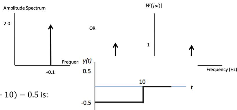
(ii) The waveform for  $y(t) = 0.5u(t - 10) - 0.5$  is:
