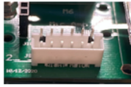
Motor connector: Straight Notches inward facing - OK
