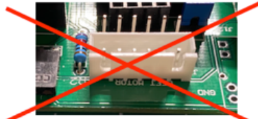
Motor connector: Straight Notches outward facing - Wrong
