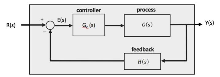
◆ The transfer function of the closed-loop control system from input R(s) to output Y(s) is (applying transforms 1 & 6):
