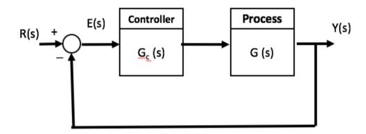
2. Adding the controller  $G_C(s)$  and closing the loop changes the system transfer function from G(s) to:
