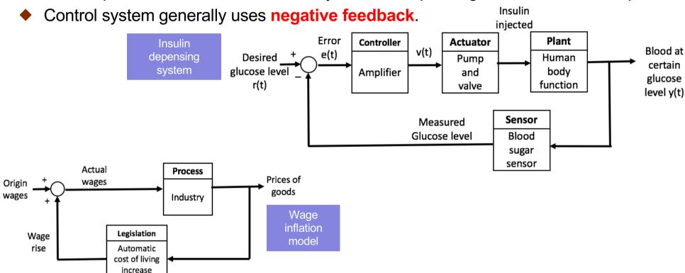
◆ A system could have **positive feedback**. Here is a model for wage inflation. Such a system will have its control parameter ever-increasing. Such a system is **not stable**, meaning that it never reaches a stable final value.
