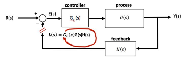
From the previous slide, we have the transfer function of a close-loop system as:
