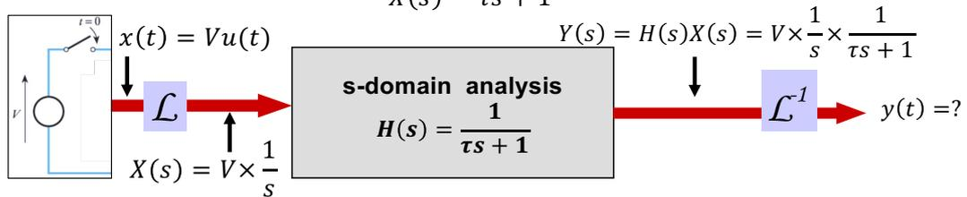
In the previous slide, we use time domain analysis and differential equations. Now let us move to the Laplace s-domain, and use Transfer function to do the same analysis. The top diagram is the time domain view of things.
