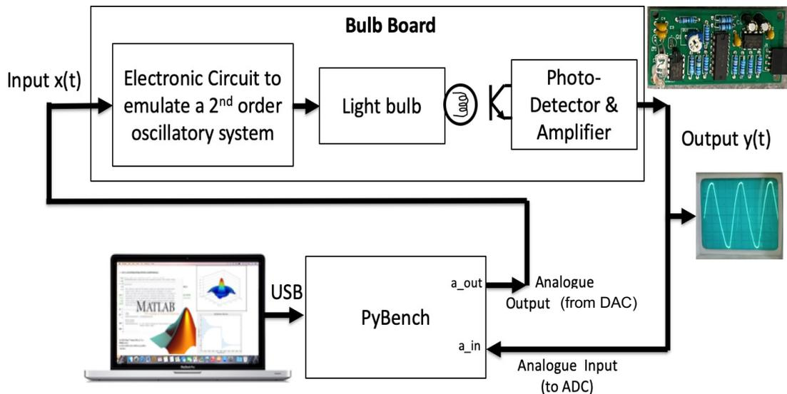
In Lab 3, you will be connecting a specially design board, called “**Bulb Board**”, to the Pybench. With Matlab, you can generate the input signal,  $x(t)$ , which is from the DAC of the Pybench to provide a stimulus signal. You can also capture the output signal,  $y(t)$  using the ADC of the Pybench. Remember, in Lab 2, you generated a sinewave and a square wave signal, and capture it back and plot the spectrum. You will be using the same system, but for a different purpose.
