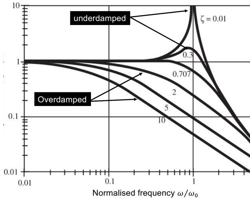
Finally, if we substitute  $s = j\omega$  into the transfer function of the second order system and compute the system gain at different frequency (the same as what you did in Lab 3, Task 2), you get the frequency response as that shown in the slide.
