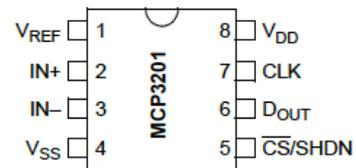
This shows the ADC block diagram we use in the Lab. Again the digital interface obeys the SPI protocol, with Chip Select (CS), Serial Clock (CLK), and Serial Data Out (Dout) signals.
