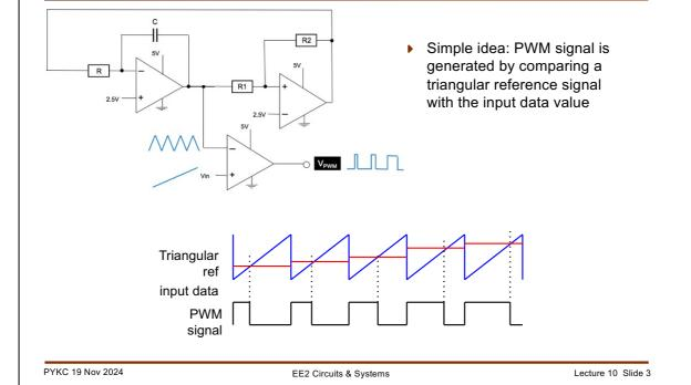
In Lecture 4, we explored the use of op-amps to build an analogue pulse-width modulator using an integrator, a comparator with hysteresis (also known as a Schmitt trigger circuit), and a simple analogue comparator.
