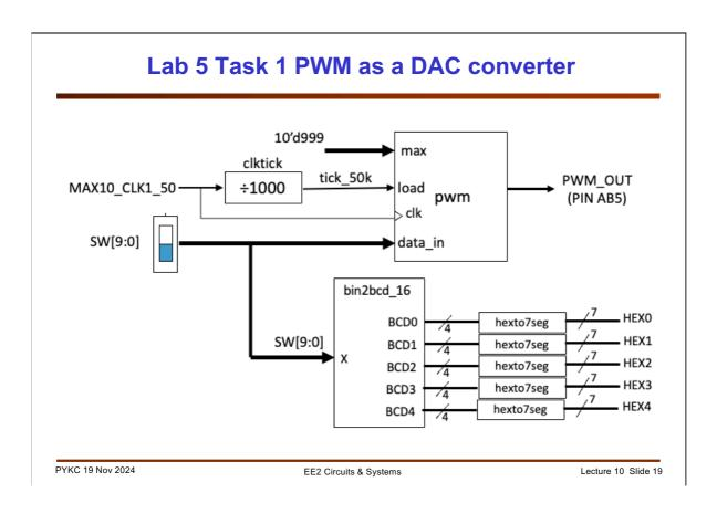
Lab 5 Task 1 is to build and test a PWM as explained in this lecture. A digital value is supplied via SW[9:0]. The pwm.v entity produces a digital output signal PWM\_OUT whose duty cycle is proportional to the digital input **data\_in**.
