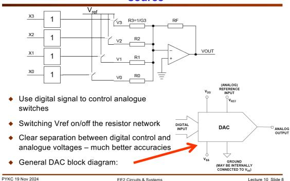
Instead of driving the resistor network directly from the digital output, which is not very accurate, most DAC actually use the digital signal to control electronic switches which switch in or out a reference voltage Vref. This reference voltage can be made very accurate, thus providing accurate output voltage values.
