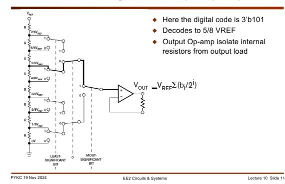
Instead of using a large number of switches, we can also use switches arranged in a tree structure as shown here. Here is an example showing the decoding of the digital value 3'b0101. Decoding is implicitly performed via the control of the switches using the three digital bits. The output op amp provides buffering of the DAC voltage.
