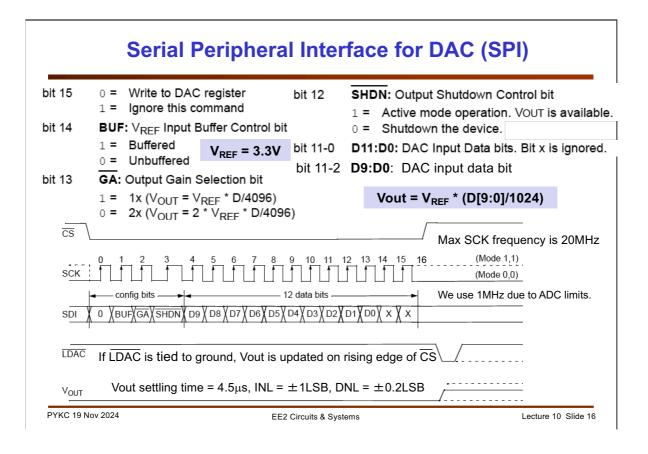
To send a value to the DAC to output (i.e. produce the analogue output Vout), a 16-bit value is sent to the DAC chip in a serial manner. The Chip Select (SC) signal going low indicate that this is the start of the data. This establishes the beginning of the data frame. First data bit (bit 15) is always 0. Bit 14 determines whether the reference voltage (Vreg) is buffered or not buffered (via an internal opamp). For our design, Vref is around 3.3V.
