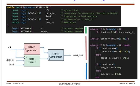
Implementing a PWM DAC is extremely simple in SystemVerilog. Here is the code with colour coding for the three major blocks.
