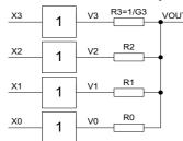
$$\begin{split} & \left(V_3 - V_{OUT}\right) G_3 + \ldots + \left(V_0 - V_{OUT}\right) G_0 = 0 \\ & V_{OUT} = \frac{V_3 G_3 + V_2 G_2 + V_1 G_1 + V_0 G_0}{G_3 + G_2 + G_1 + G_0} \\ & R_{Thevenin} = \frac{1}{G_3 + G_2 + G_1 + G_0} \end{split}$$
