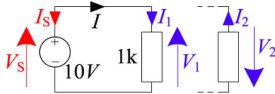
$$P_R = V_1 \times I_1 = (+10) \times (+0.01) = +0.1 \text{ W}$$
