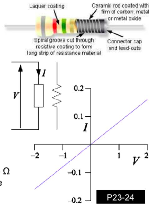
The most basic component in electronics is the resistor. Its value, the resistance  $R$  provides the simple relationship between voltage and current through Ohm's law.
