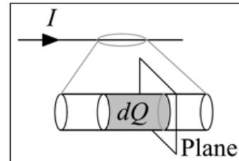
$I = -1 \text{ A} \Rightarrow 1 \text{ C}$  of +ve charge in the direction **opposite** to the arrow.
