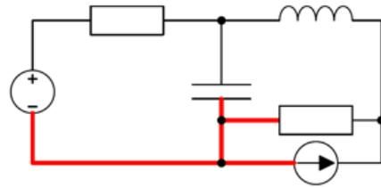
A **node** in a circuit is all the points that are connected together via the interconnecting wires. One of the four nodes in the diagram is coloured red.
