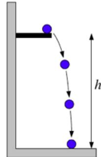
The potential energy difference between any two points is the energy needed to move 1 kg from one point to the other.
