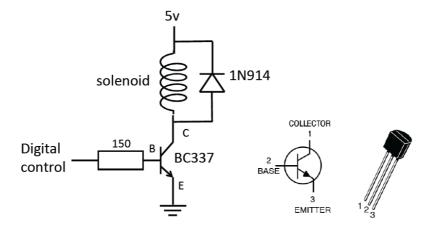
The digital output from the Pyboard delivers is about 20mA at 3.3V when it outputs a '1'. The voltage across the base-emitter of the NPN bipolar transistor is around 0.7V when the transistor is ON. Therefore the current flowing into the transistor's base terminal is around 17mA.
