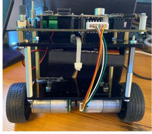
However, if you are to attempt self-balancing, it is easier to balance if the centre of gravity is higher up. For this reason, you may want to attach the battery as high as possible.
