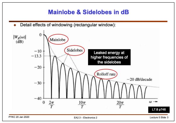
Let us examine the magnitude spectrum of the rectangular function (in dB). It has a main region where most of the energy lies. This is call the mainlobe of the spectrum. In addition, energy is also spread to its neighbouring lobes, the sidelobes. This is known as "leakages" — energy leaked from the main frequency component.
