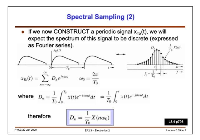
When you use the Matlab function fft(sig) to compute the spectral component values, you perform the Discrete Fourier Transform (DFT) calculation using a fast algorithm. The fast algorithm is known as Fast Fourier Transform. How this is done is not important. It is sufficient to know that a straight calculation of DFT on a N sample signal has a computation complexity of order(N²). Using FFT, we reduce this order(N log N). Say, if N 1000, using FFT instead of DFT would be over 300 times faster!
