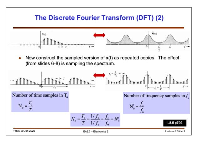
The most important message of this slide is how to work out  $N_0$  and  $T_0$  for a given sampling frequency fs (sampling period T = 1/fs).
