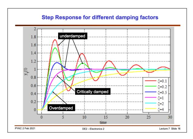
For a second order system, the unit step response is shown here for different value of  $\zeta$  .
