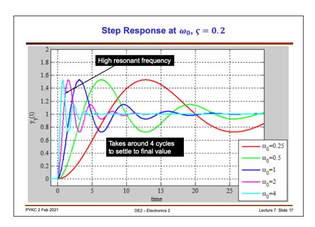
Now let us fix  $\zeta$  = 0.2 and change the resonant frequency  $\omega_0$ . Note that the time it takes for the signal to reach (nearly) the final value is related to the number of cycles of oscillation.
