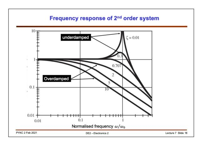
Finally, if we substitute s = jw into the transfer function of the second order system and compute the system gain at different frequency (the same as what you did in Lab 3, Task 2), you get the frequency response as that shown in the slide.
