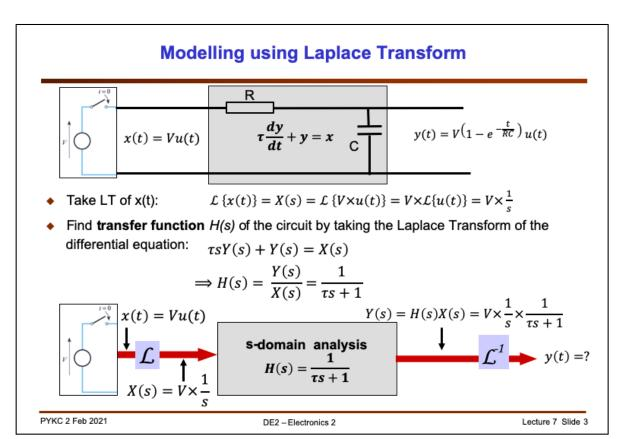
In the previous slide, we use time domain analysis and differential equations. Now let us move to the Laplace s-domain, and use Transfer function to do the same analysis. The top diagram is the time domain view of things.
