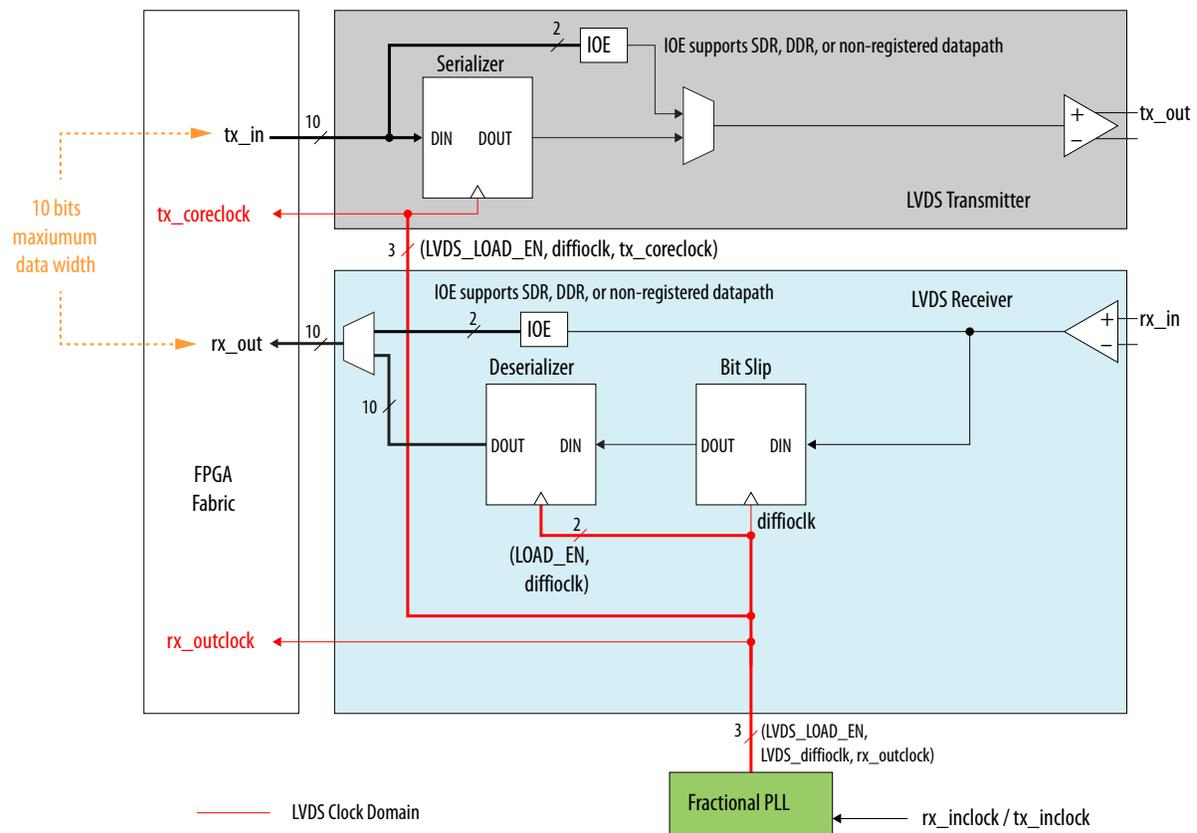
The preceding figure shows a shared PLL between the transmitter and receiver. If the transmitter and receiver do not share the same PLL, you require two fractional PLLs. In single data rate (SDR) and double data rate (DDR) modes, the data width is 1 and 2 bits, respectively.
