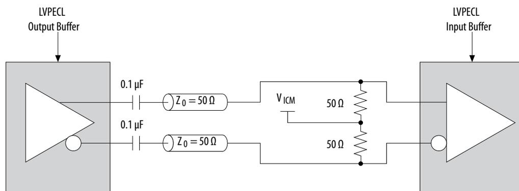
Support for DC-coupled LVPECL is available if the LVPECL output common mode voltage is within the Cyclone V LVPECL input buffer specification.
