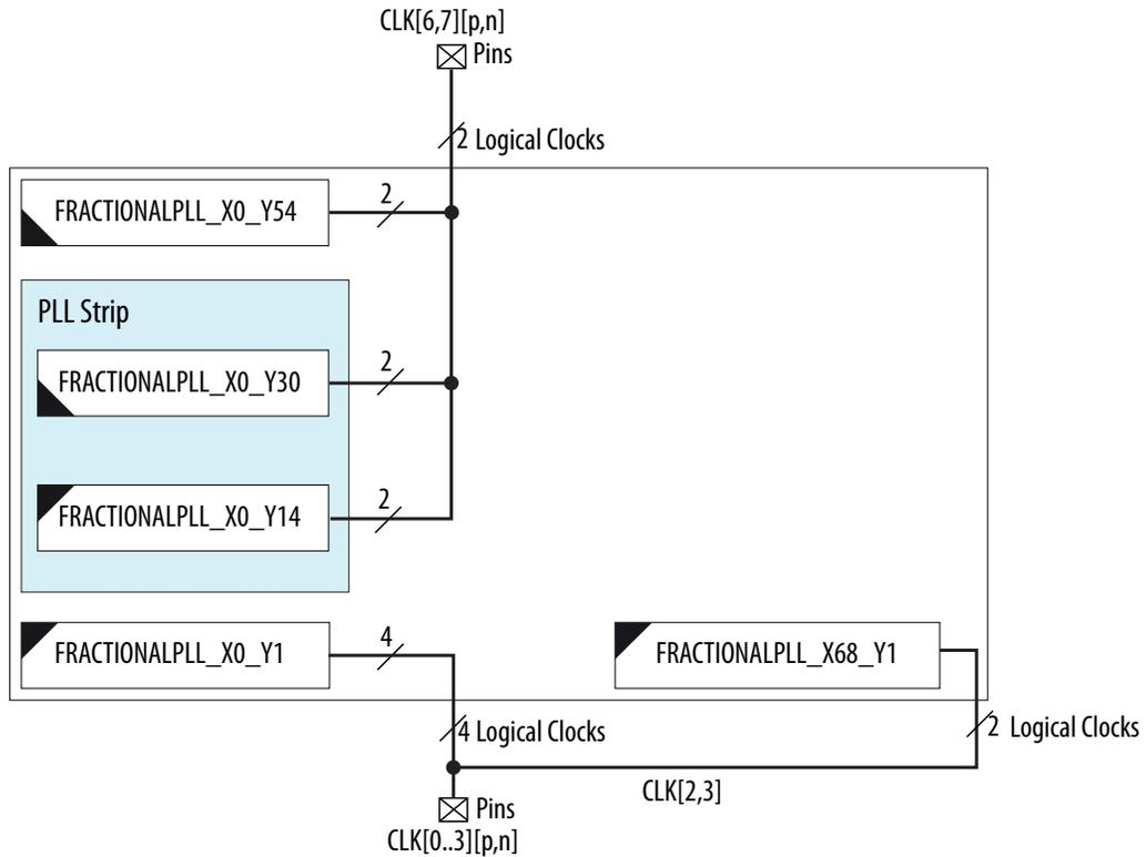
**Figure 4-22: PLL Locations for Cyclone V SE A5 and A6 Devices, Cyclone V SX C5 and C6 Devices, and Cyclone V ST D5 and D6 Devices**
