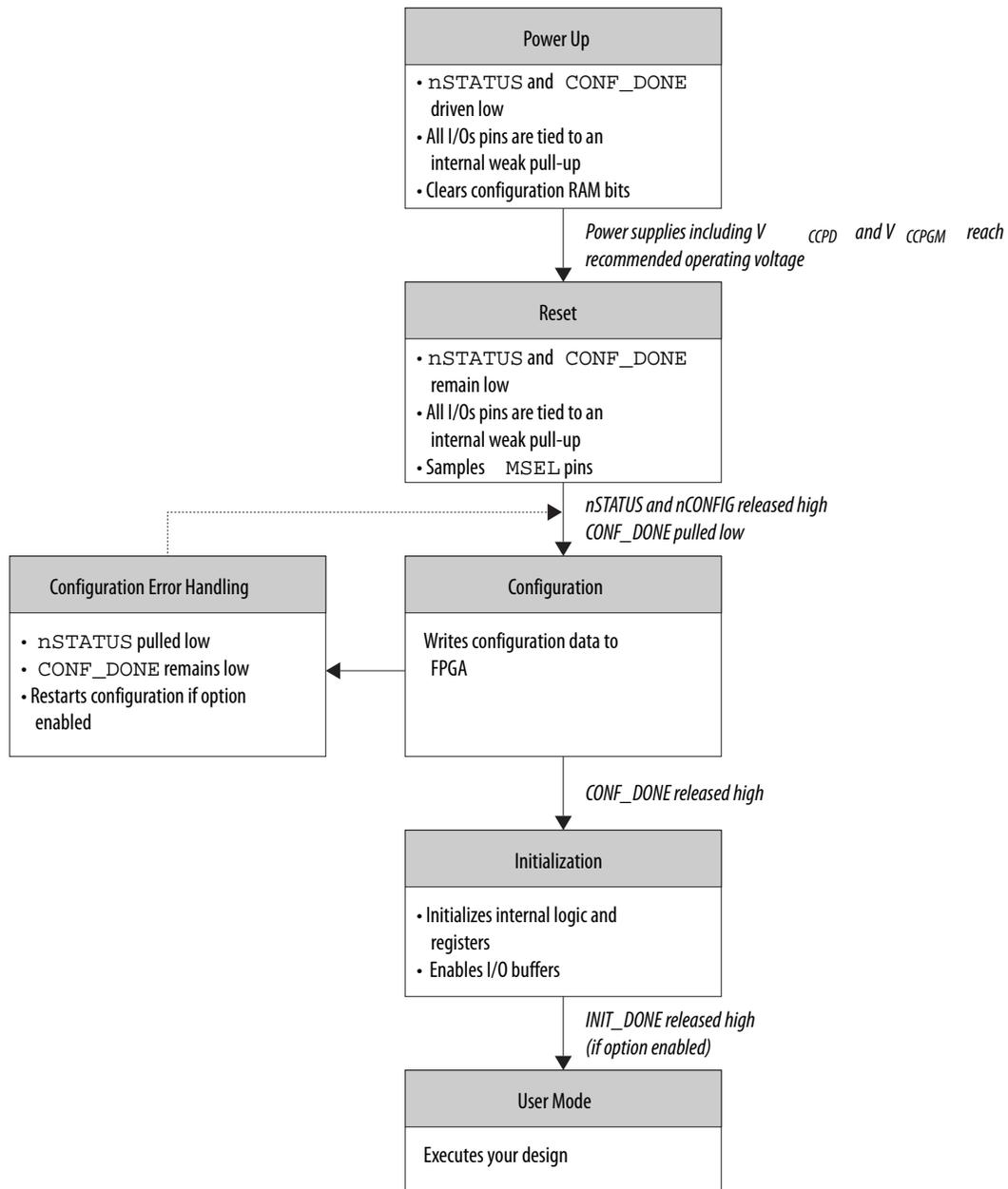
You can initiate reconfiguration by pulling the  $nCONFIG$  pin low to at least the minimum  $t_{CFG}$  low-pulse width except for configuration using the partial reconfiguration operation. When this pin is pulled low, the  $nSTATUS$  and  $CONF\_DONE$  pins are pulled low and all I/O pins are tied to an internal weak pull-up.
