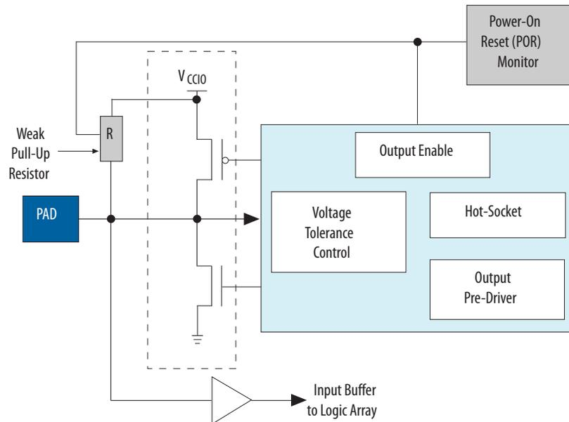
The POR circuitry monitors the voltage level of the power supplies and keeps the I/O pins tri-stated until the device is in user mode. The weak pull-up resistor (R) in the Cyclone V input/output element (IOE) is enabled during configuration download to keep the I/O pins from floating.
