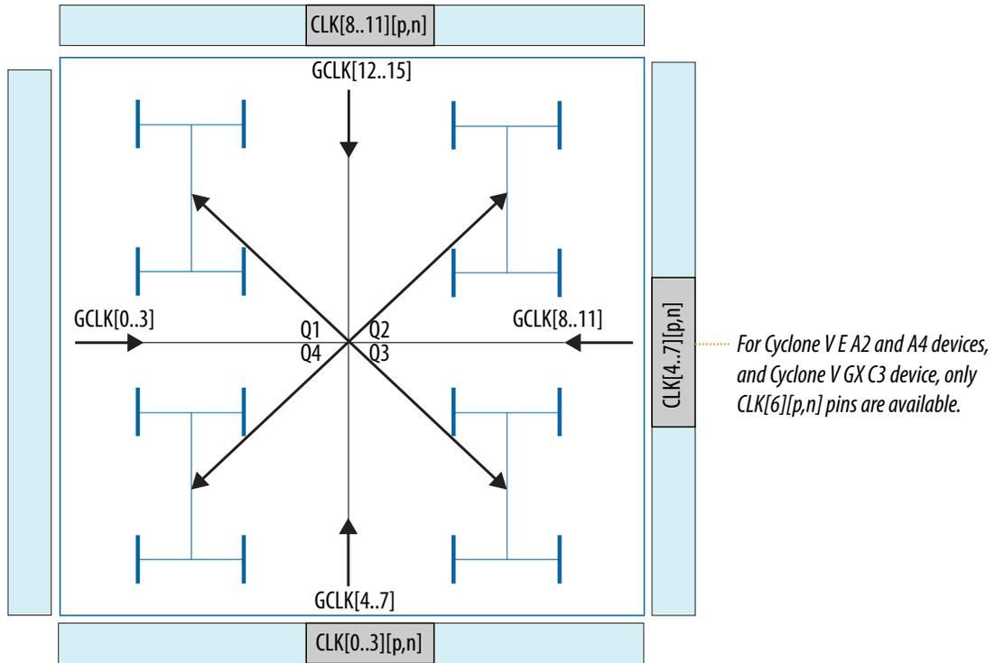
**Figure 4-2: GCLK Networks in Cyclone V SE, SX, and ST Devices**
