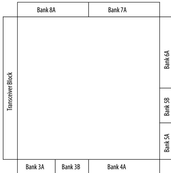
Figure 5-8: I/O Banks for Cyclone V SE Devices
