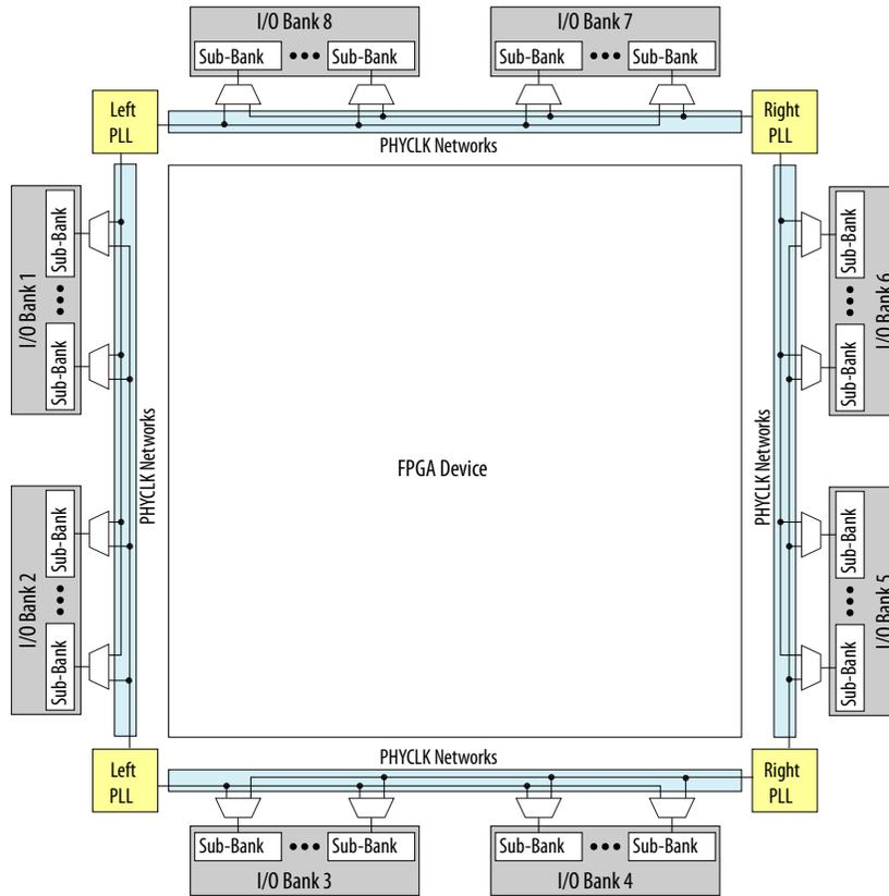
Figure 6-9: PHYCLK Networks in Cyclone V GX C3 Devices
