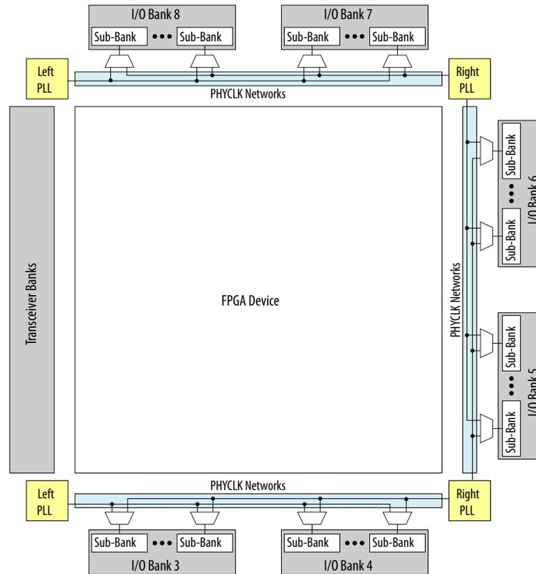
Figure 6-11: PHYCLK Networks in Cyclone V SE A2, A4, A5, and A6 Devices
