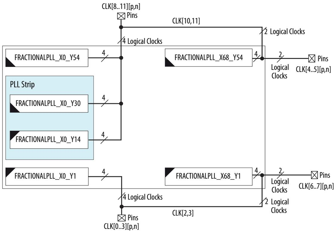
**Figure 4-19: PLL Locations for Cyclone V E A7 Device, Cyclone V GX C7 Device, and Cyclone V GT D7 Device**
