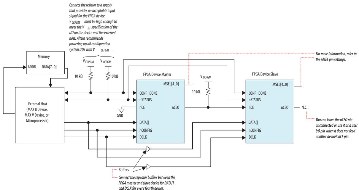
When a device completes configuration, its nCEO pin is released low to activate the nCE pin of the next device in the chain. Configuration automatically begins for the second device in one clock cycle.
