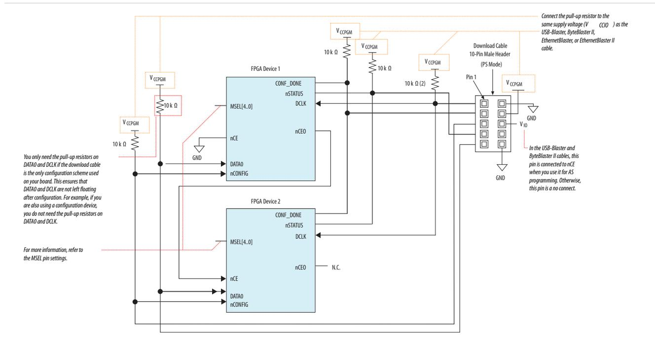
When a device completes configuration, its nCEO pin is released low to activate the nCE pin of the next device. Configuration automatically begins for the second device.
