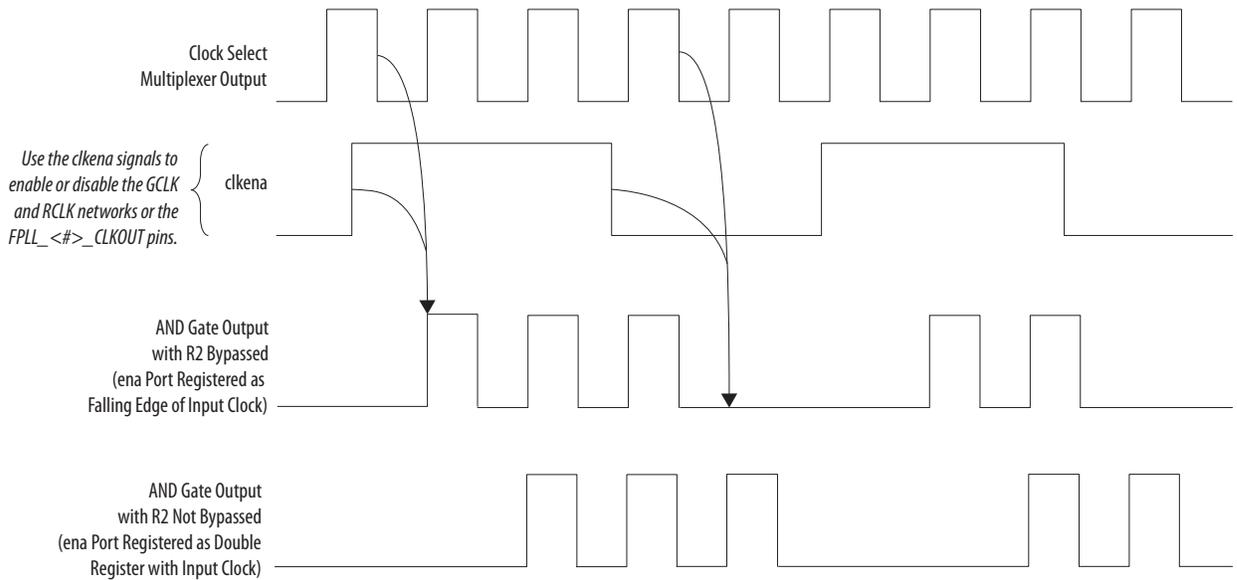
Cyclone V devices have an additional metastability register that aids in asynchronous enable and disable of the GCLK and RCLK networks. You can optionally bypass this register in the Quartus Prime software.
