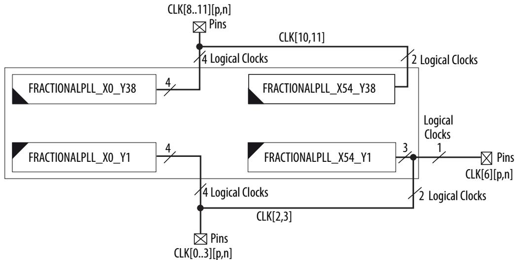
**Figure 4-17: PLL Locations for Cyclone V GX C3 Device**
