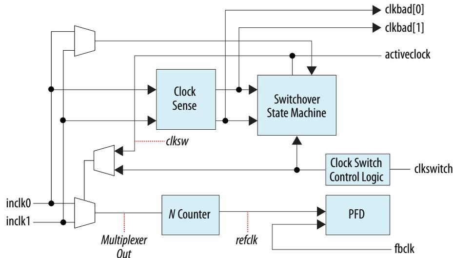
When the current reference clock is not present, the clock sense block automatically switches to the backup clock for PLL reference. You can select a clock source as the backup clock by connecting it to the `inclk1` port of the PLL in your design.
