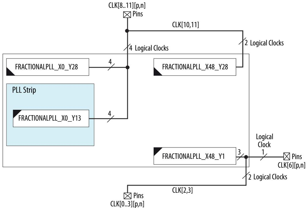
**Figure 4-18: PLL Locations for Cyclone V E A5 Device, Cyclone V GX C4 and C5 Devices, and Cyclone V GT D5 Device**
