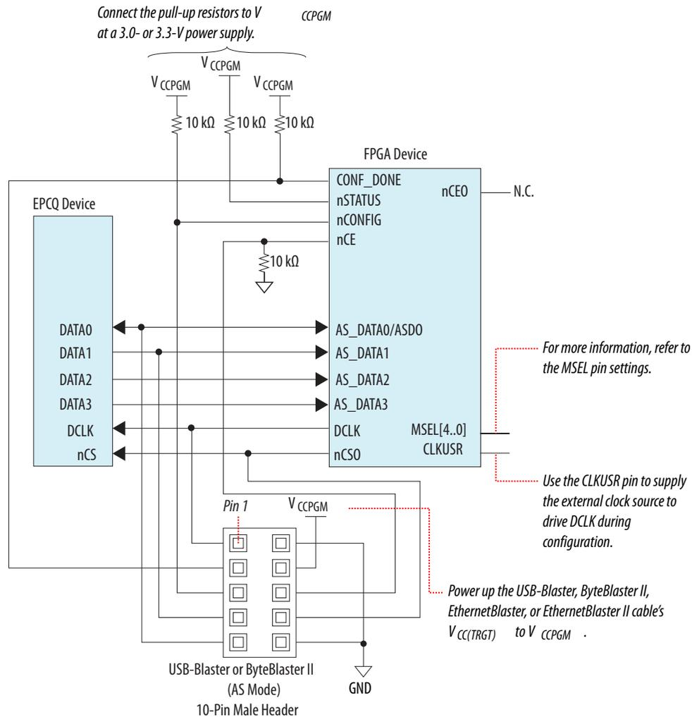
When programming the EPCS and EPCQ devices, the download cable disables access to the AS interface by driving the `nCE` pin high. The `nCONFIG` line is also pulled low to hold the Cyclone V device in the reset stage. After programming completes, the download cable releases `nCE` and `nCONFIG`, allowing the pull-down and pull-up resistors to drive the pin to GND and  $V_{CCPGM}$ , respectively.
