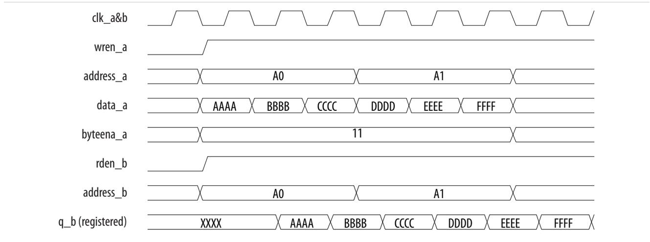
**Figure 2-4: Mixed-Port Read-During-Write: Old Data Mode**
