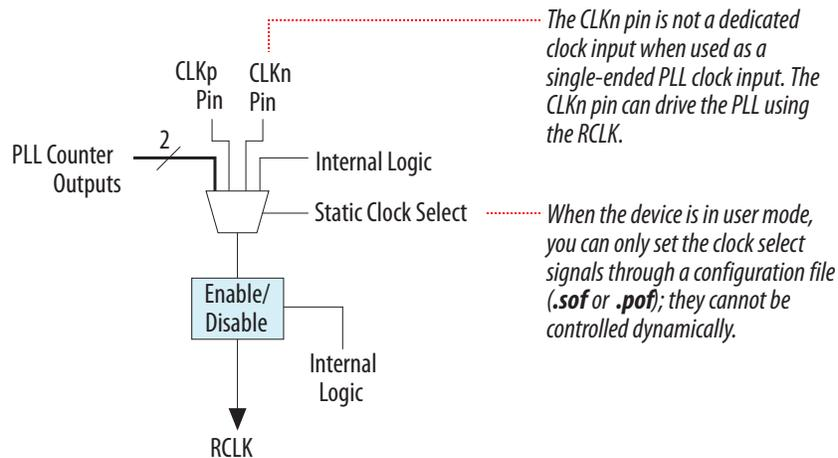
You can set the input clock sources and the `clkena` signals for the GCLK and RCLK network multiplexers through the Quartus Prime software using the ALTCLKCTRL IP core.
