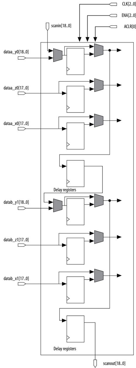
**Figure 3-3: Input Register of a Variable Precision DSP Block in 27 x 27 Mode for Cyclone V Devices**
