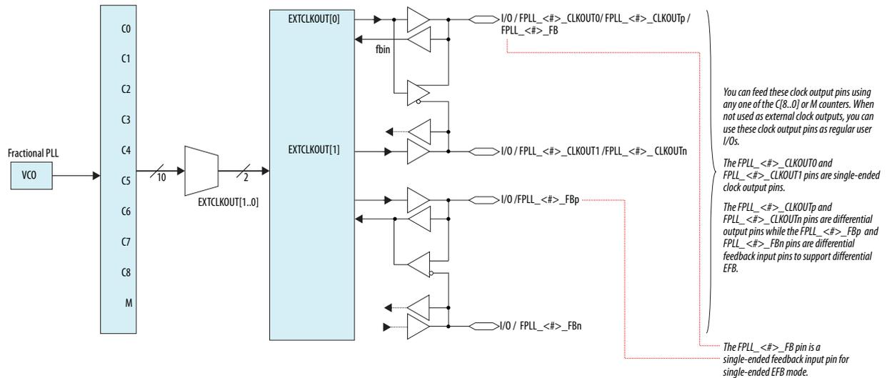
Each pin of a single-ended output pair can be either in-phase or 180° out-of-phase. To implement the 180° out-of-phase pin in a pin pair, the Quartus Prime software places a NOT gate in the design into the IOE.
