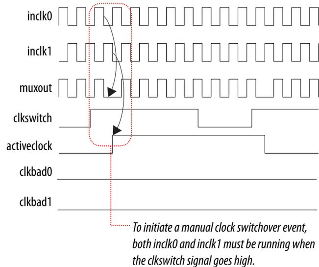
In automatic override with manual switchover mode, the `activeclock` signal mirrors the `clkswitch` signal. Since both clocks are still functional during the manual switch, neither `clkbad` signal goes high. Because the switchover circuit is positive-edge sensitive, the falling edge of the `clkswitch` signal does not cause the circuit to switch back from `inclk1` to `inclk0`. When the `clkswitch` signal goes high again, the process repeats.
