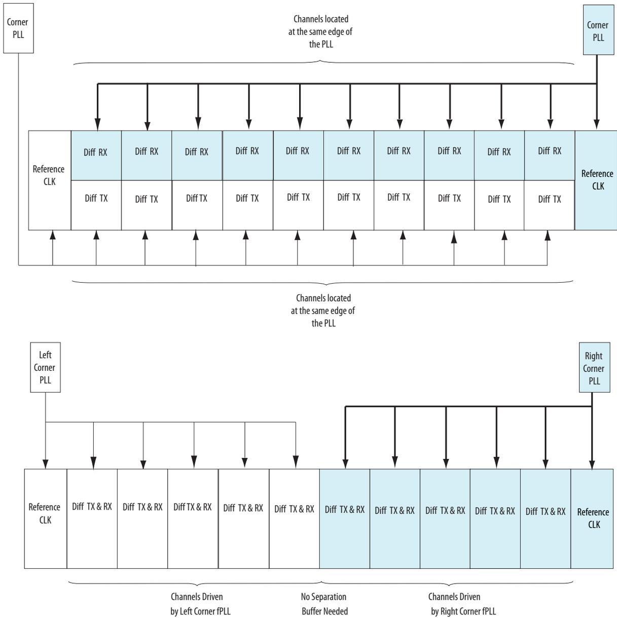
**Figure 5-3: Invalid Placement of Differential I/Os Due to Interleaving of Channels Driven by the Corner PLLs**
