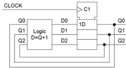
The logic block must add 1 onto the current value of the counter, Q, to generate the next value of the counter, D. Suppose it has a propagation delay of 1ns.
