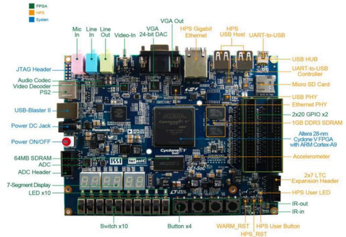
The practical aspects of this course module is based around a FPGA board, the DE1-SoC. Here is an overall block diagram of the board. Don't worry about the details for now. I will be explaining to you the various bits on the board later when you are about to start the VERI experiment in the Lab in mid-November.
