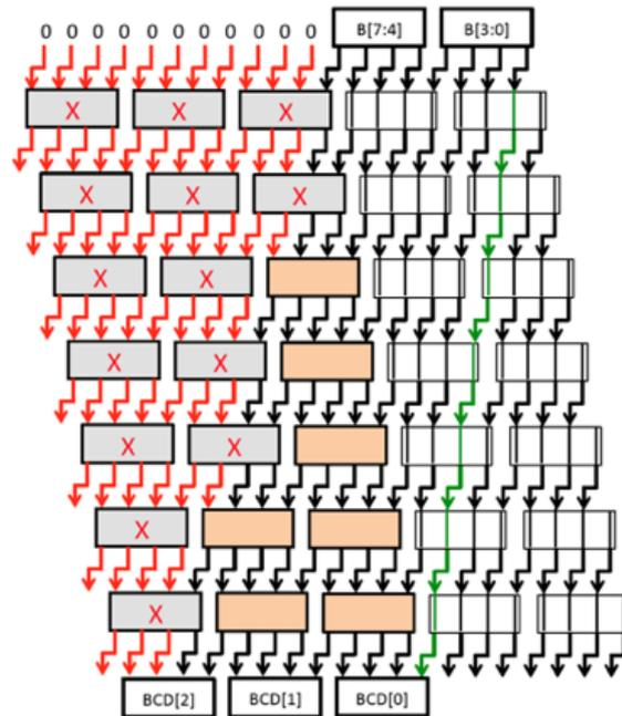
The full array is more complicated than need be. If we propagate the '0's forward in the array of gates, you will find those marked with 'X' will always have its input less than 5. In which, **output = input** in these modules. THIS IS JUST A SET OF FOUR WIRES.
