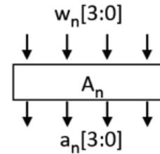
Assuming that we have designed a module “**add3\_ge5**” to perform the adjustment as required, the converter can be implemented in Verilog by simply “WIRING UP” the various modules together.
