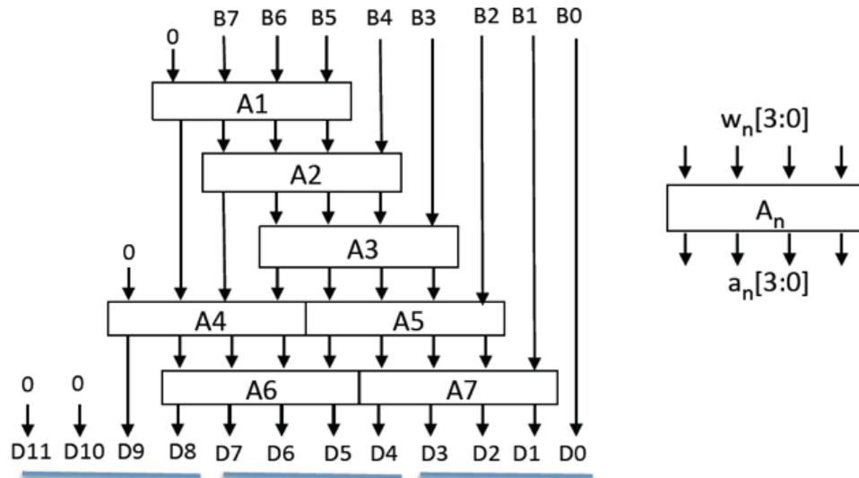
After simplification, here are ALL the remaining **add3\_ge5** modules for the 8-bit binary to BCD conversion (bin2bcd8). I have labeled the input ports to **add3\_ge3**  $w_n[3:0]$  and the output parts  $a_n[3:0]$  where n is 1 to 7.
