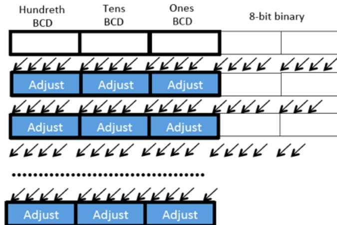
In order to understand how to we may implement this converter in hardware, you have to understand that shifting in hardware is easy. You just need to connect signals with one bit shift to the left. It DOES NOT need any gates, just wires!
