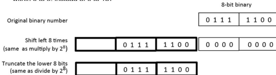
Before we examine this algorithm in detail, let us consider the arithmetic operation of shifting left by one bit. This is the same as a  $\times 2$  operation.
