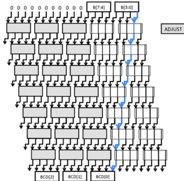
The entire full array is shown here. The shade module is the adjust module (which we call: **add3\_ge5**).
