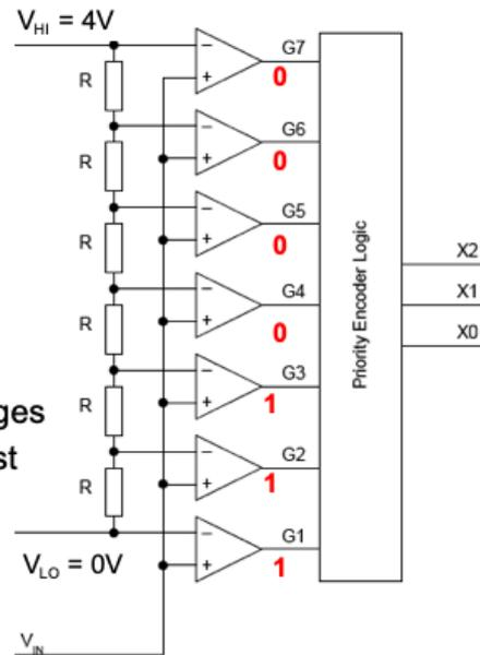
The simplest ADC is the flash ADC. We are converting from the range of 0V to 4V to a digital range of 0 to 7 in binary.
