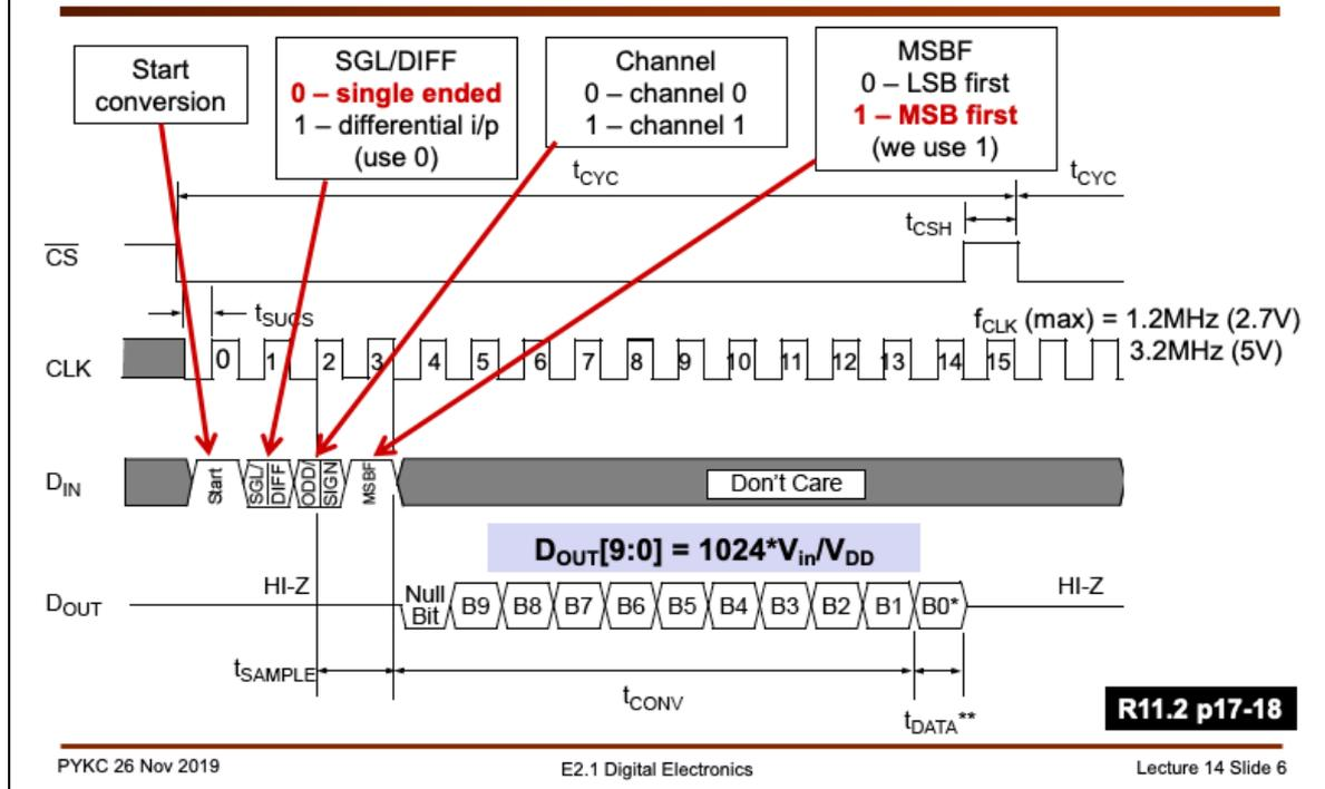
The control of the ADC is slightly more complicated than that for the DAC. Nevertheless, the idea is similar. The transfer cycle is again 16 states, going from state 0 to state 15.
