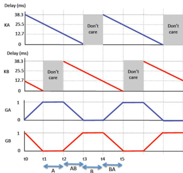
Finally, with minor modifications to the processing module, using TWO delay components and a variable gain (with time), it is possible to produce a pitch changer. There will not be enough time during the experiment for you to do this part. However, it may be a suitable Christmas project.
