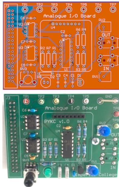
I also provide a purpose-built ADC/DAC board to support the lab experiment. This add-on board is only needed in week 3 onwards during the laboratory sessions. So for now, you can ignore it.
