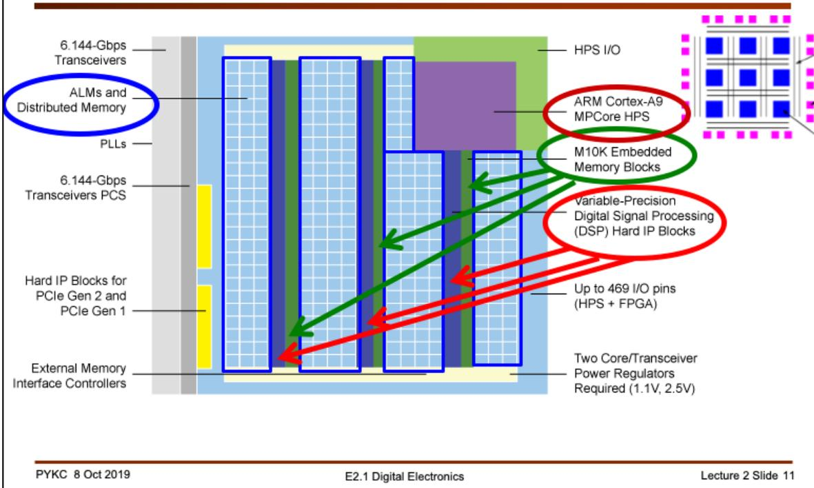
The Cyclone V is much more than just an FPGA with a bunch of Logic Elements (or ALMs). Our chip in the DE1 board has 32,000 ALMs, which is around 85K old style 4-input LUT LEs. On top of that, it also has over 4Mbit of embedded memory, 87 DSP blocks (to do multiply-accumulate operations needed for signal processing), and even a dual-core ARM microprocessor!
