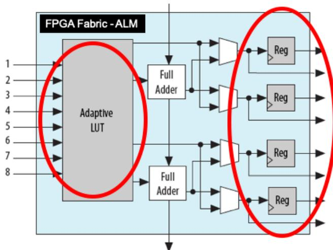
Let us now look at the FPGA that you will use for this course. The Altera Cyclone V FPGA has a more advanced programmable logic element than the simple 4-input LUT that we have considered up to now. They call this an Adaptive Logic Module or ALM.
