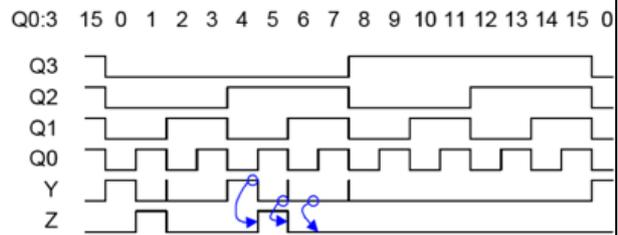
Eliminating glitches can be achieved by adding an extra D-FF at Y output. Z will be glitch free. However, **beware that Z is one cycle delayed relative to Y.**
