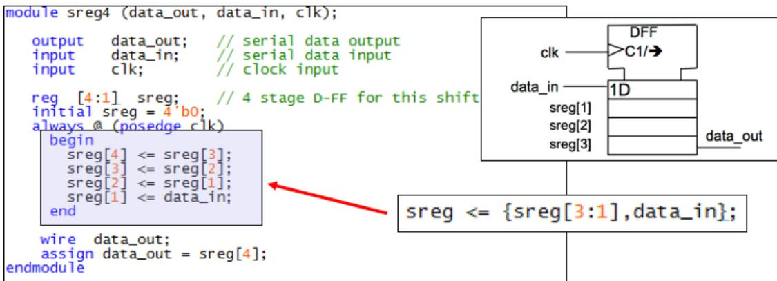
To specify a shift register in Verilog, use the code shown here (in blue box). We use the `<=` assignment to make sure that `sreg[4:1]` are updated only at the end of the `always` block.
