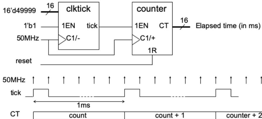
Using this style of designing a clock tick circuit allows us to easily connect multiple counters in series as shown here.
