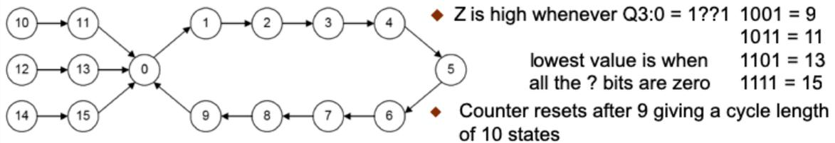
What if you want a counter that only counts from 0 to 9, then back to 0 again? This is really easy with Verilog. A simple if-else construct testing for the terminal counter of 9 will do the trick.
