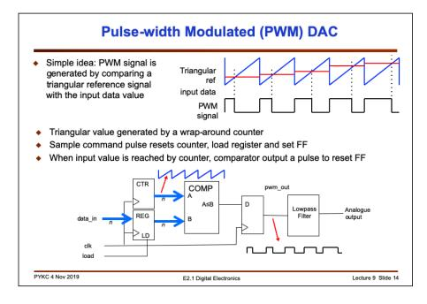
Instead of using analogue resistor network, it is possible to build a simple DAC using only digital components.
