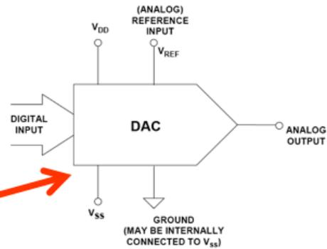
Instead of driving the resistor network directly from the digital output, which is not very accurate, most DAC actually use the digital signal to control electronic switches which switch in or out a reference voltage  $V_{ref}$ . This reference voltage can be made very accurate, thus providing accurate output voltage values.
