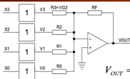
$$V_{OUT} = \frac{-R_F}{R_{Thévenin}} \times V_{Thévenin} = -R_F (V_3 G_3 + V_2 G_2 + V_1 G_1 + V_0 G_0)$$
