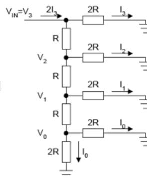
String resistor network is good for, say, up to 10-bit DAC (requiring 1024 identical resistors). If you want a 16-bit DAC, you would need 65536 resistors! That is obviously not practical or too expensive. A better solution is to use R-2R Ladder network.
