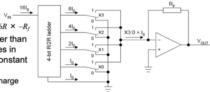
For a practical DAC circuit, the R/2R ladder network is connected to the virtual earth of the op amp as shown here. The current is either sent to the virtual earth node if the digital value is '1', or switched to earth if it is '0'. In that way, the output voltage  $V_{out}$  is a converter analogue value of  $X_{3:0}$ .
