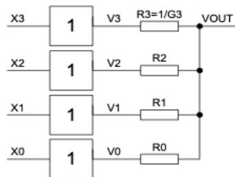
$$(V_3 - V_{OUT})G_3 + \dots + (V_0 - V_{OUT})G_0 = 0$$
