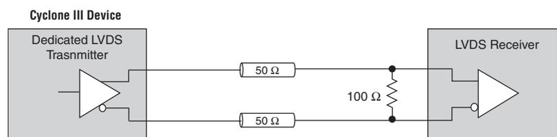
Figure 8-4 shows the LVDS I/O interface with external resistor network on the top and bottom I/O banks.
