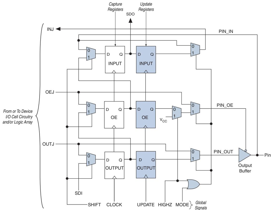
Table 14-3 describes the capture and update register capabilities of all boundary-scan cells within Cyclone III devices.
