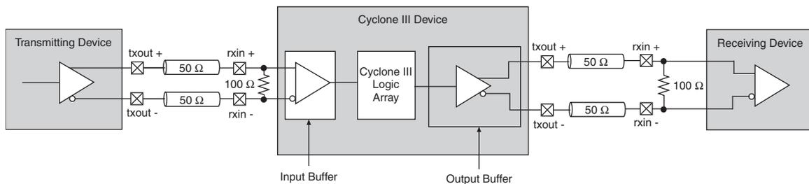
Figure 8-3 shows the LVDS I/O interface with dedicated output buffer on the left and right I/O banks.
