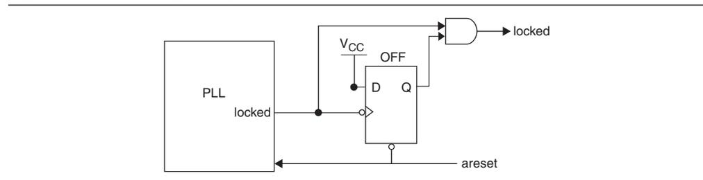
If you use the SignalTap® II tool to probe the `locked` signal before the D flipflop, the `locked` signal goes low only when `areset` is deasserted. If the `areset` signal is not enabled, the extra logic is not implemented in the ALTPLL megafunction.
