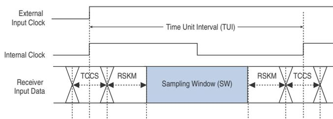
Figure 8–26 shows the Cyclone III high-speed I/O timing budget.
