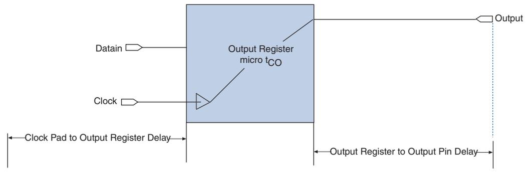
The Quartus II software reports the  $t_{CO}$  timing with the conditions shown in Table 1-39 using the above equation.
