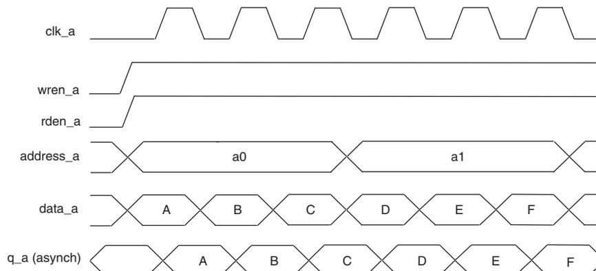
**Figure 4-24.** Same Port Read-During-Write: Old Data Mode
