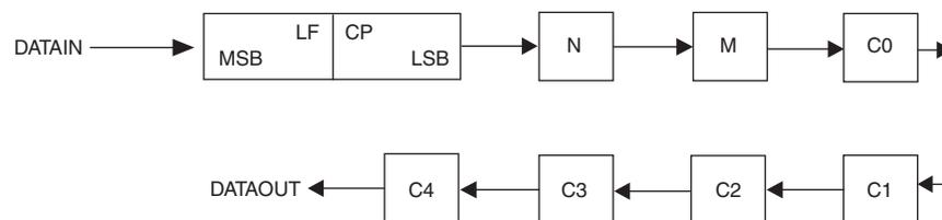
Figure 6-28 shows the scan chain bit order sequence for one PLL post-scale counter in Cyclone III PLLs.
