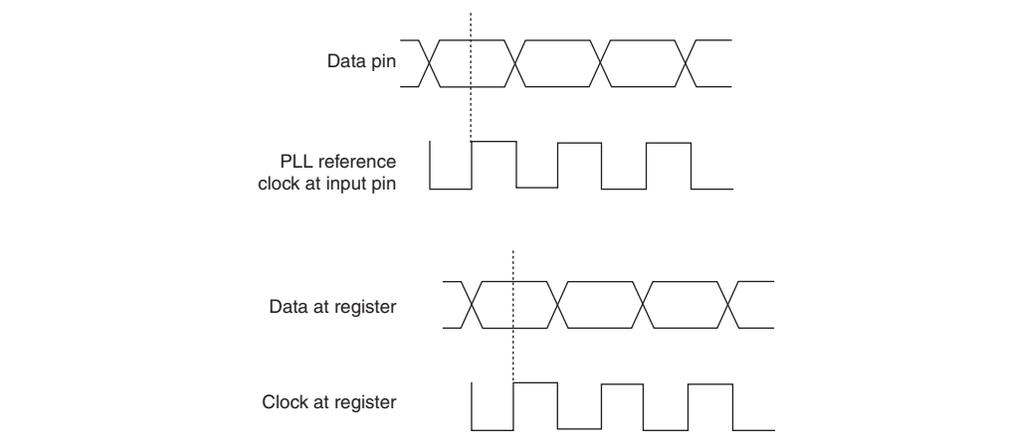
Source-synchronous mode compensates for delay of the clock network used plus any difference in the delay between these two paths:
