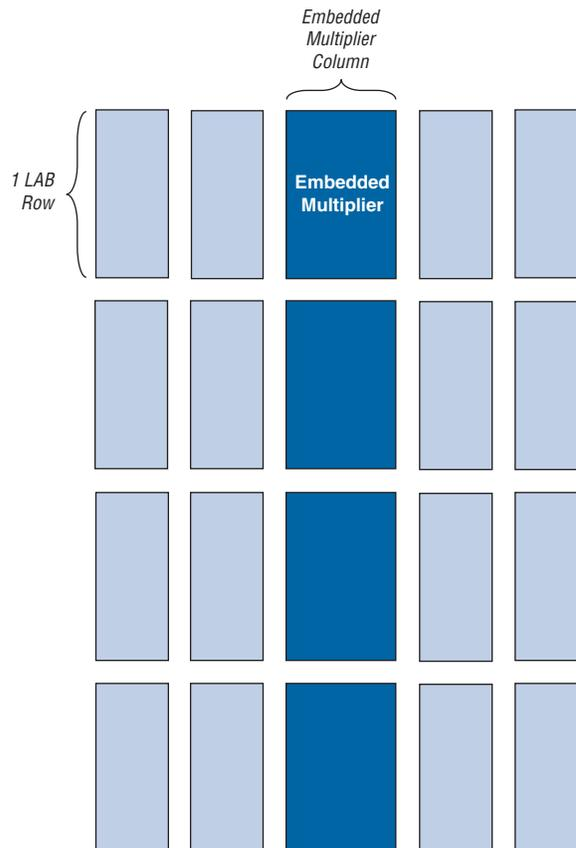
The number of embedded multipliers per column and the number of columns available increases with device density.
