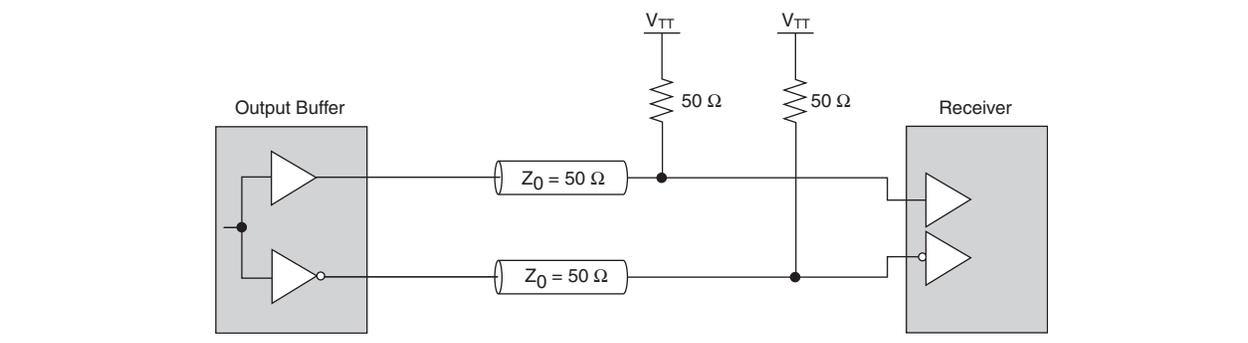
**Figure 8-23.** Differential HSTL Class II Interface
