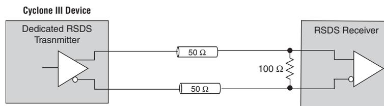
**Figure 8-10.** RSDS Interface with External Resistor Network on the Top and Bottom I/O Banks (Note 1)
