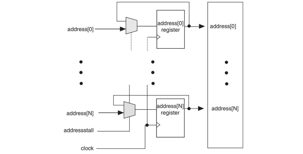
The address clock enable is typically used for cache memory applications to improve efficiency during a cache-miss. The default value for the address clock enable signals is low.
