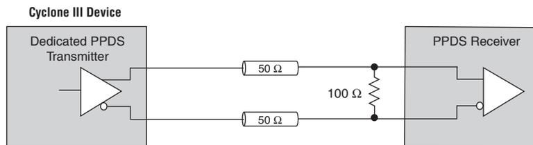
**Figure 8-17.** PPDS Interface with External Resistor Network on the Top and Bottom I/O Banks
