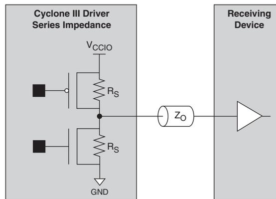
All I/O banks and I/O pins support impedance matching and series termination. Dedicated configuration pins and JTAG pins do not support impedance matching or series termination.
