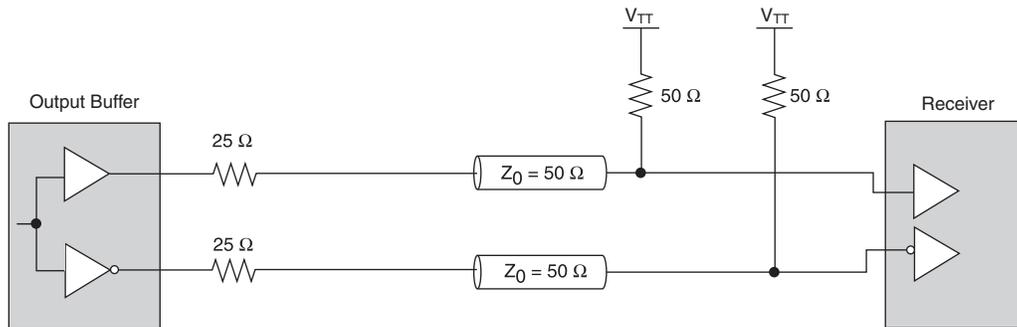
**Figure 8-21.** Differential SSTL Class II Interface
