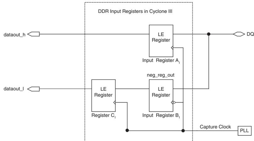
The DDR data is first fed to two registers, input register A<sub>1</sub> and input register B<sub>1</sub>.
