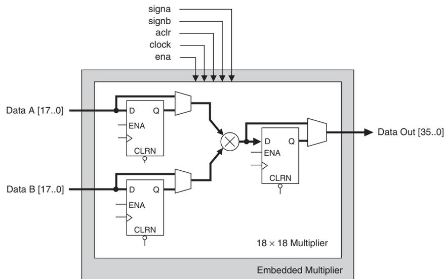
All 18-bit multiplier inputs and results can be sent independently through registers. The multiplier inputs can accept signed integers, unsigned integers, or a combination of both. Additionally, you can change the *signa* and *signb* signals dynamically and send these signals through dedicated input registers.
