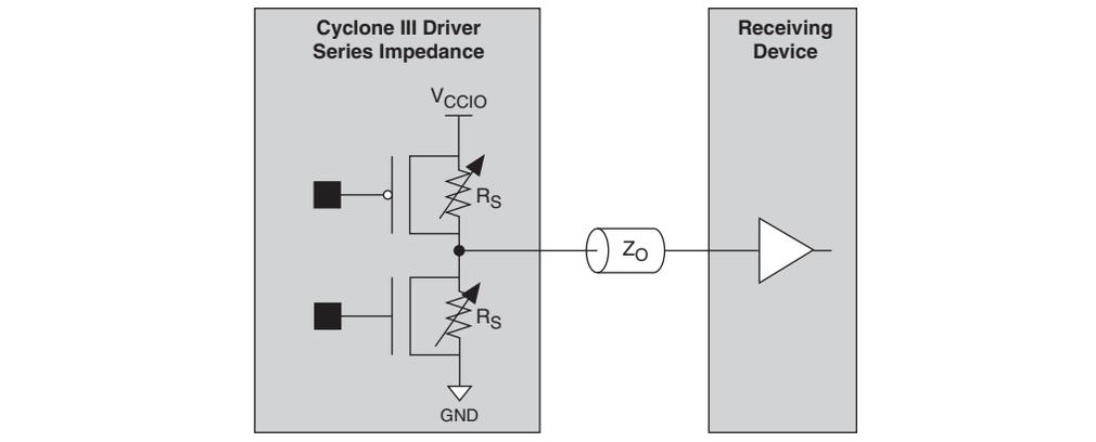
OCT with calibration is achieved using the OCT calibration block circuitry. There is one OCT calibration block in banks 2, 4, 5, and 7. Each calibration block supports each side of the I/O banks. Because there are two I/O banks sharing the same calibration block, both banks must have the same  $V_{CCIO}$  if both banks enable OCT calibration. If two related banks have different  $V_{CCIO}$ s, only the bank where the calibration block resides can enable OCT calibration.
