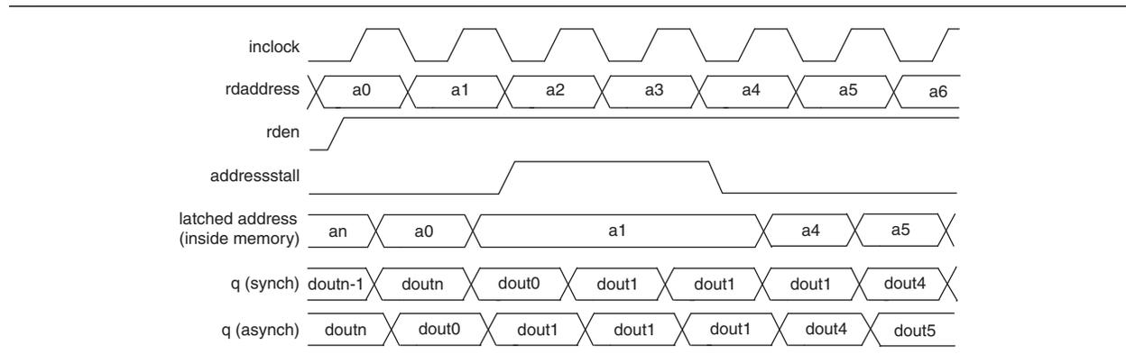
**Figure 4-5.** Cyclone III Address Clock Enable During Write Cycle Waveform
