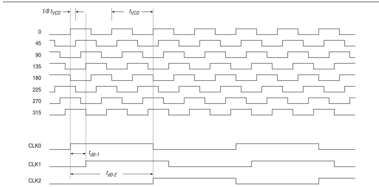
You can use the coarse and fine phase shifts to implement clock delays in Cyclone III devices.
