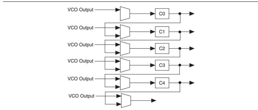
When cascading counters to implement a larger division of the high-frequency VCO clock, the cascaded counters behave as one counter with the product of the individual counter settings.
