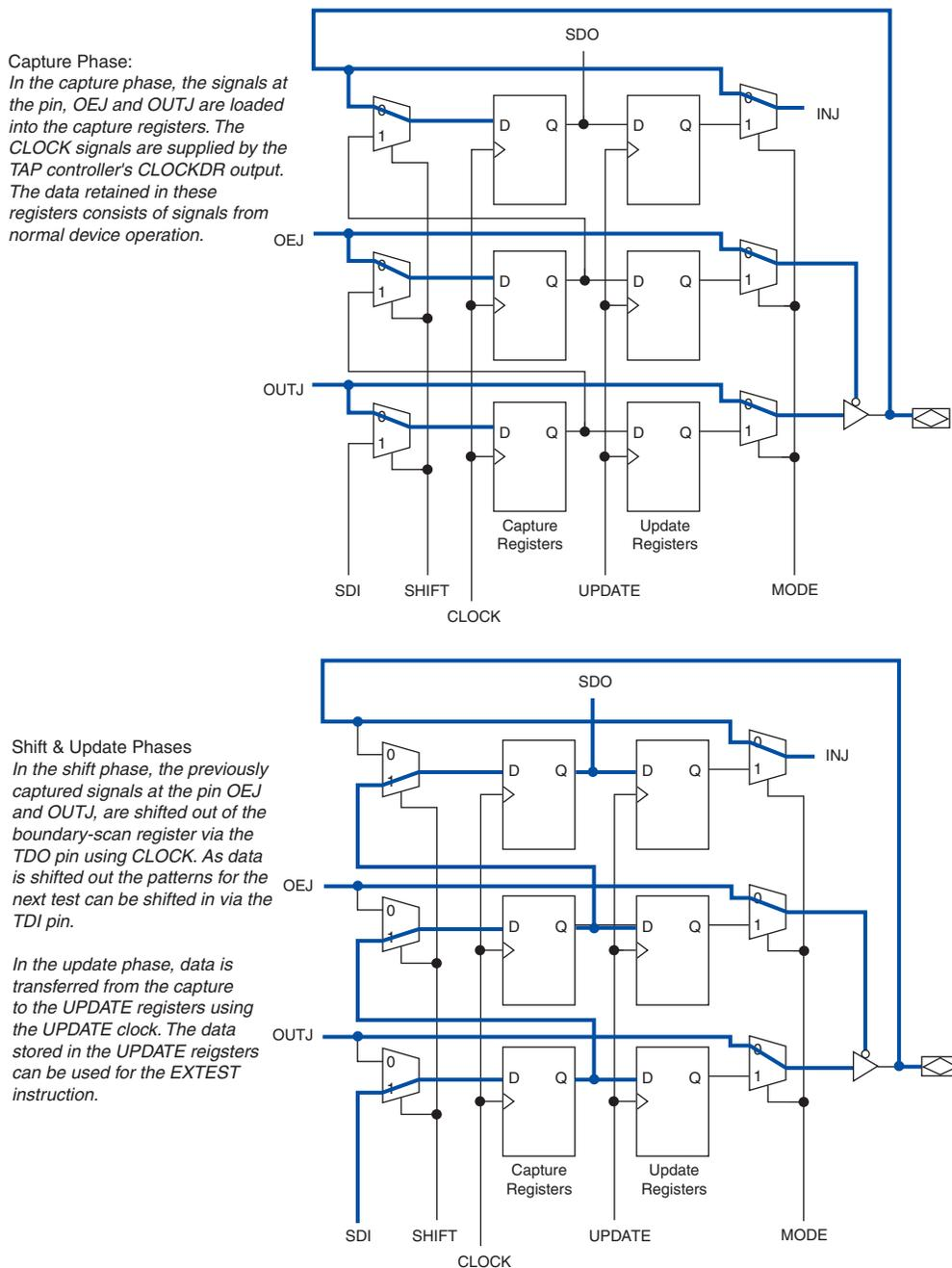
During the capture phase, multiplexers preceding the capture registers select the active device data signals. This data is then clocked into the capture registers. The multiplexers at the outputs of the update registers also select active device data to prevent functional interruptions to the device. During the shift phase, the boundary-scan shift register is formed by clocking data through capture registers around the
