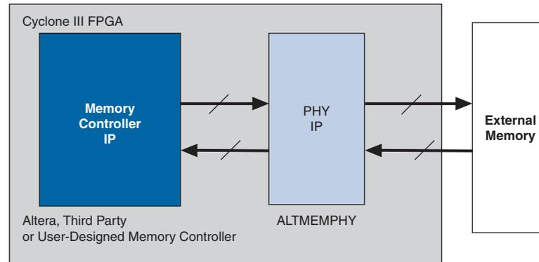
This chapter includes a description of the hardware interfaces for external memory interfaces available in the Cyclone III devices.
