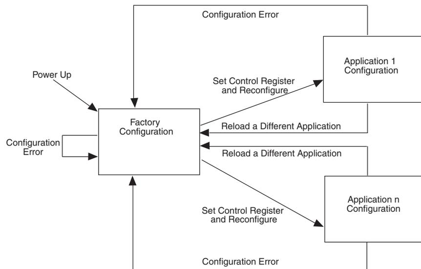
After power up or a configuration error, the factory configuration logic writes the remote system upgrade control register to specify the address of the application configuration to be loaded. The factory configuration also specifies whether or not to enable the user watchdog timer for the application configuration and, if enabled, specify the timer setting.
