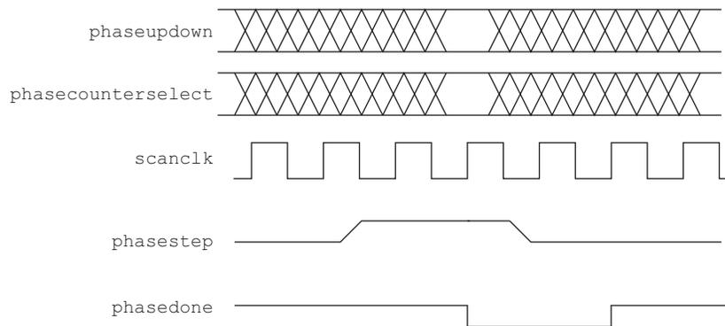
Depending on the VCO and scanclk frequencies, phasedone low time may be greater than or less than one scanclk cycle. The maximum time for reconfiguring phase shift dynamically is to be determined (TBD) based on device characterization.
