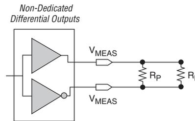
**Figure 1-6.** Output Delay Timing Reporting Setup Modeled by Quartus II Software for Differential Outputs with Three External Resistor Network
