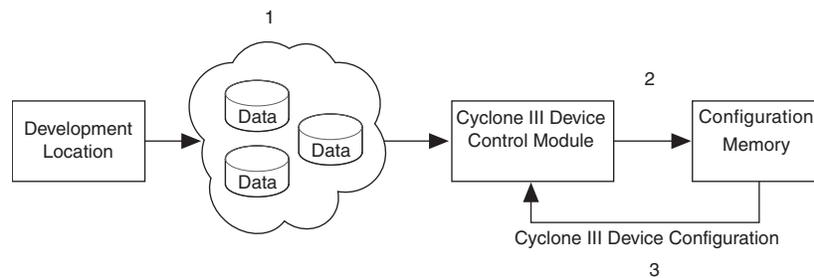
Cyclone III devices only support remote system upgrade in the AS and AP configuration schemes. Remote system upgrade can also be implemented in conjunction with advanced Cyclone III features such as real-time decompression of configuration data in an AS configuration scheme.
