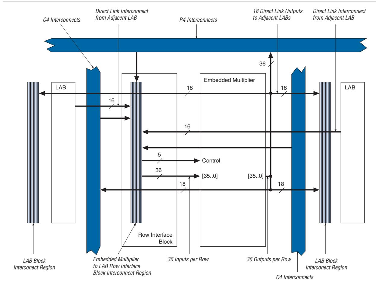
There are five dynamic control input signals that feed the embedded multiplier:
