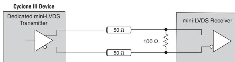
**Figure 8-14.** mini-LVDS Interface with External Resistor Network on the Top and Bottom I/O Banks (Note 1)
