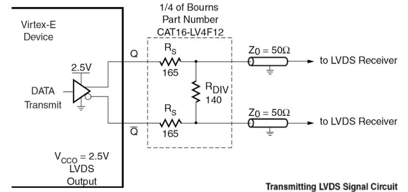
Transmitting LVDS Signal Circuit
