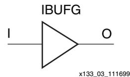
Figure 3: Virtex Global Clock Input Buffer Symbol (IBUFG)
