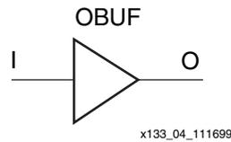
Figure 4: Virtex Output Buffer Symbol (OBUF)
