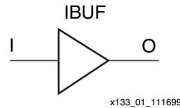
Figure 1: Input Buffer Symbol (IBUF)
