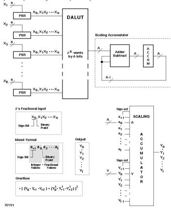
Fig. 3. Serially Organized DA processor
