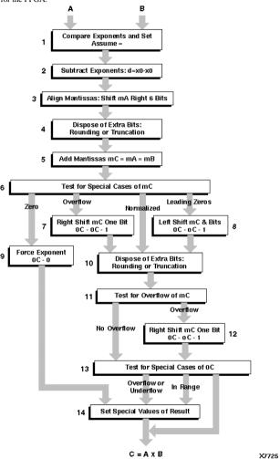
Fig. 5a. Floating-Point Addition
