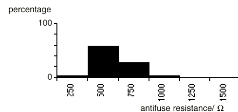
The resistance of blown Actel antifuses
